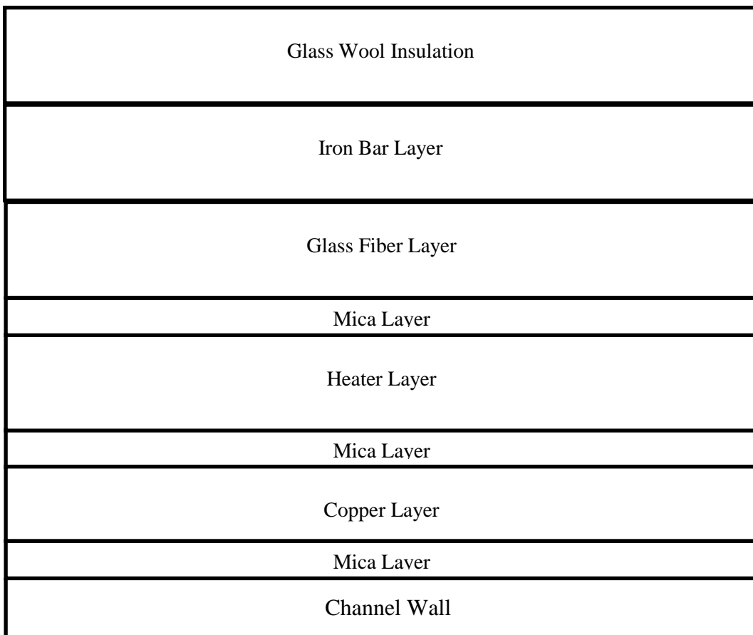
Figure 3.9 Heating layer model (not to scale)
