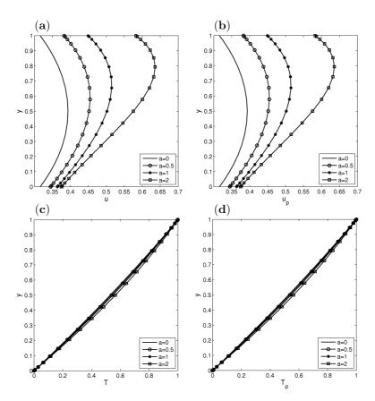
Figure 3.23: Problem 3.4: Steady-state solutions when Ha = 1, b = 0.01 and  $\beta = 1$  for different viscosity parameter a: (a) u, (b)  $u_p$ , (c) T, (d)  $T_p$ .
