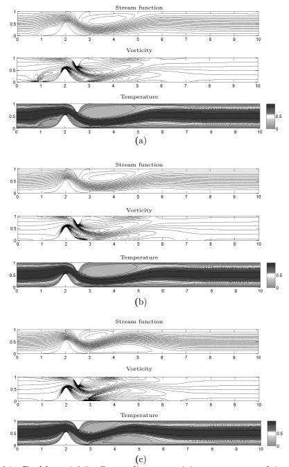
Figure 4.24: Problem 4.6.5: Streamlines, vorticity contours and isotherms for Re = 100,  $Mn_F = 82$ ,  $Mn_M = 0.025$ , (a) a = 1.0, (b) a = 2.5, (c) a = 3.0.
