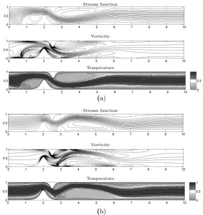
Figure 4.25: Problem 4.6.5: Streamlines, vorticity contours and isotherms, Re = 100,  $Mn_F = 656$ ,  $Mn_M = 1.2$ : (a) a = 1.0, (b) a = 3.0.
