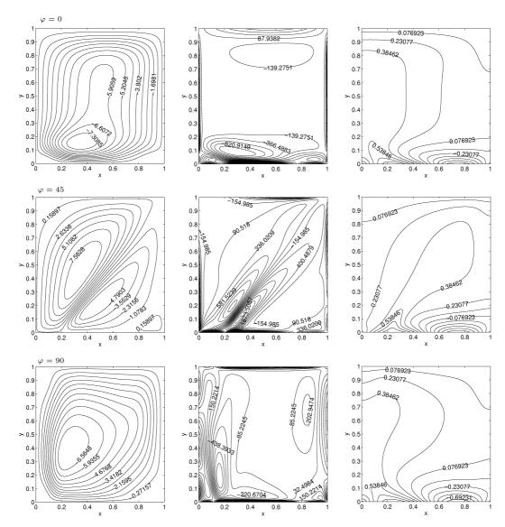
Figure 2.16: Problem 2.4.4.1: Streamlines (L), vorticity contours (M) and isotherms (R) when  $Ra = 10^6$  and Ha = 100 for  $\phi = 0$ ,  $\varphi = 0$ , 45 and 90.
