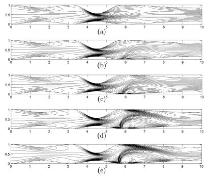
Figure 4.30: Problem 4.6.6: Vorticity contours for Re=100: (a)  $Mn_F=0$ ,  $Mn_M=0$ , (b)  $Mn_F=82$ ,  $Mn_M=0.025$ , (c)  $Mn_F=164$ ,  $Mn_M=0.1$ , (d)  $Mn_F=656$ ,  $Mn_M=1.2$ , (e)  $Mn_F=1312$ ,  $Mn_M=6.4$ .
