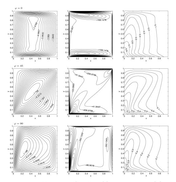
Figure 2.23: Problem 2.4.4.2: Streamlines (L), vorticity contours (M) and isotherms (R) when  $Ra=10^6$  and Ha=100 for  $\phi=-45,~\varphi=0,~45$  and 90.
