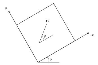
Figure 1.1: Problem geometry and the coordinate system for natural convection flow.
