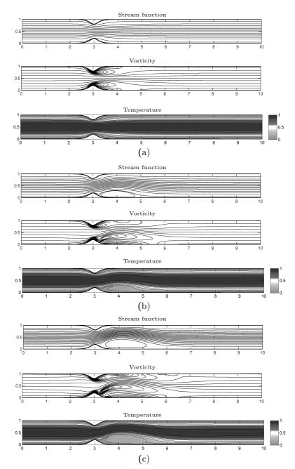
Figure 4.17: Problem 4.6.4: Streamlines, vorticity contours and isotherms 40% stenosis for Re=100, (a)  $Mn_F=Mn_M=0$ , (b)  $Mn_F=82$ ,  $Mn_M=0.025$ , (c)  $Mn_F=164$ ,  $Mn_M=0.1$ .
