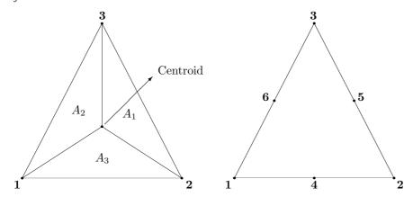
Figure 2.1: Three-nodal (linear) and six-nodal (quadratic) triangular elements.
