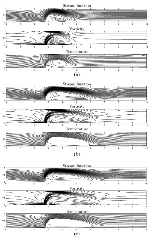
Figure 4.10: Problem 4.6.2: Time evaluation of stream function, vorticity and temperature contours for  $Re=100,\ Mn=1312$  when (a)  $t=0.2,\ (b)\ t=1.0,\ (c)\ t=5.0.$
