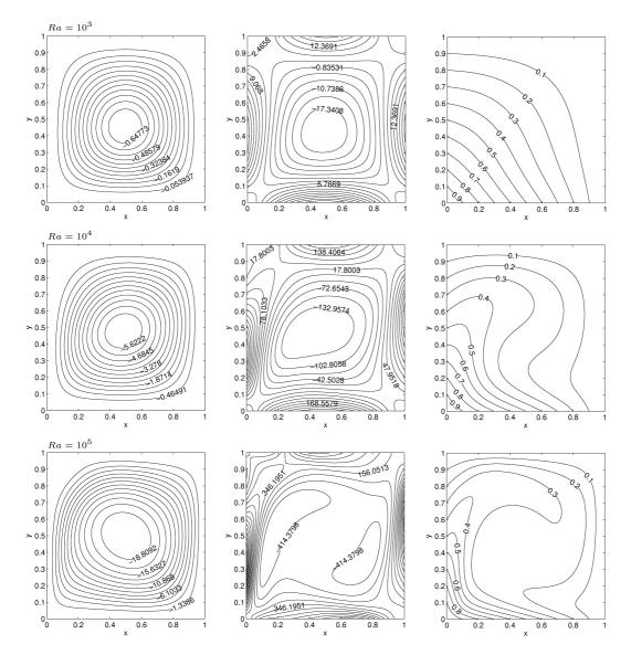
Figure 2.18: Problem 2.4.4.2: Streamlines (L), vorticity contours (M) and isotherms (R) when Ha=0 for  $Ra=10^3$ ,  $10^4$  and  $10^5$ ,  $\phi=0$ ,  $\varphi=0$ .
