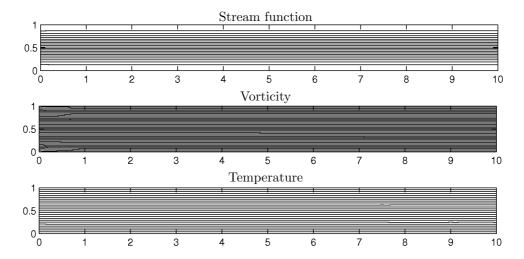
Figure 4.7: Problem 4.6.1: Streamlines, vorticity contours and isotherms (FEM) for Re = 250, Mn = 0.
