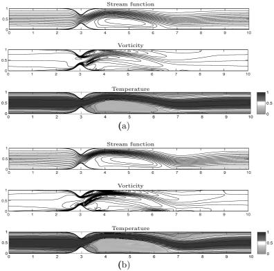
Figure 4.19: Problem 4.6.4: Streamlines, vorticity contours and isotherms 60% stenosis for Re = 100, (a)  $Mn_F = 656$ ,  $Mn_M = 1.2$ , (b)  $Mn_F = 1312$ ,  $Mn_M = 6.4$ .
