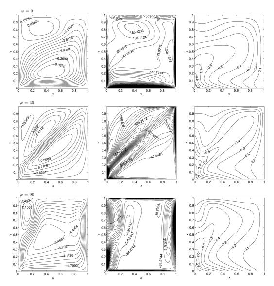
Figure 2.21: Problem 2.4.4.2: Streamlines (L), vorticity contours (M) and isotherms (R) when  $Ra=10^6$  and Ha=100 for  $\phi=0,\,\varphi=0,\,45$  and 90.
