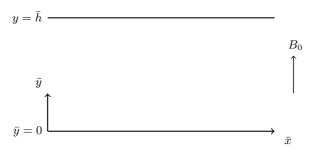
Figure 1.3: Problem configuration for MHD flow of a dusty fluid.
