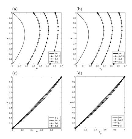
Figure 3.25: Problem 3.4: Steady-state solutions when Ha = 1, a = 1 and b = 0.01 for different Navier-slip parameter  $\beta$ : (a) u, (b)  $u_p$ , (c) T, (d)  $T_p$ .
