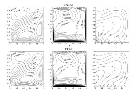
Figure 3.9: Problem 3.2.3: Streamlines (L), vorticity (M) and temperature (R) contours for  $Ra=10^6$  and  $Ha=100, \phi=0, \varphi=0$ .
