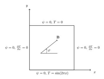
Figure 2.13: The geometry and boundary conditions of Problem 2.4.4.1.
