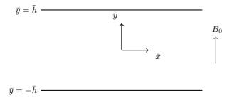
Figure 1.2: Problem configuration for MHD flow between parallel plates.
