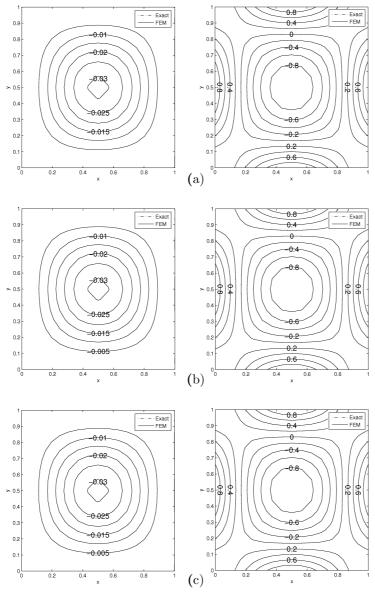
Figure 3.3: Problem 3.2.1: Streamlines (L) and vorticity contours (R) when N=24 for (a) Re=0, (b)  $Re=10^3$ , (c)  $Re=10^4$ .
