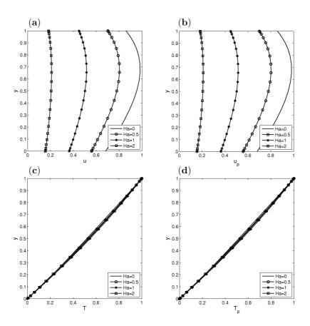
Figure 3.26: Problem 3.4: Steady-state solutions when  $a=1,\,b=0.01$  and  $\beta=1$  for different Hartmann numbers: (a)  $u,\,$  (b)  $u_p,\,$  (c)  $T,\,$  (d)  $T_p.$
