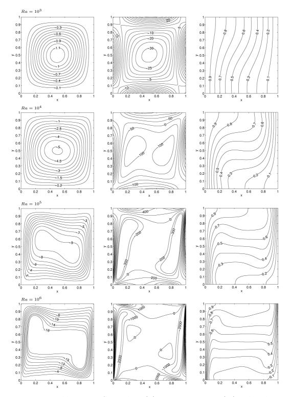
Figure 2.12: Problem 2.4.3: Streamlines (L), vorticity contours (M) and isotherms (R) for  $Ra=10^3,\ 10^4,\ 10^5$  and  $10^6.$
