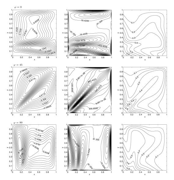
Figure 2.22: Problem 2.4.4.2: Streamlines (L), vorticity contours (M) and isotherms (R) when  $Ra=10^6$  and Ha=100 for  $\phi=45,\,\varphi=0,\,45$  and 90.
