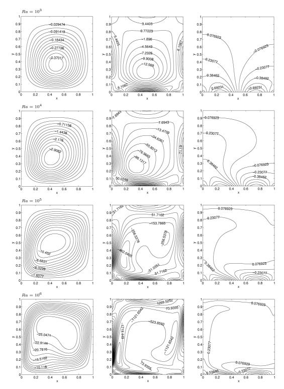
Figure 2.14: Problem 2.4.4.1: Streamlines (L), vorticity contours (M) and isotherms (R) for Ha = 10,  $Ra = 10^3$ ,  $10^4$ ,  $10^5$  and  $10^6$ .
