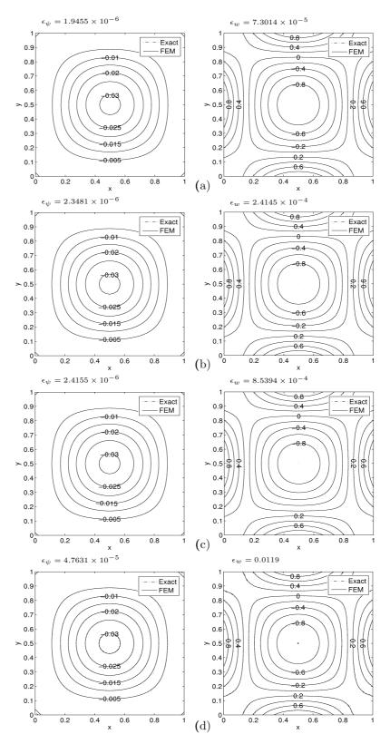
Figure 2.6: Problem 2.4.1: Streamlines (L) and vorticity contours (R) for (a) Re = 0, (b)  $Re = 10^3$ , (c)  $Re = 10^4$ , (d)  $Re = 10^6$ .
