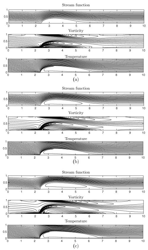
Figure 4.8: Problem 4.6.1: Effects of magnetic field on streamlines, vorticity contours and isotherms (FEM) for Re=250,  $(a)\,Mn=115$ ,  $(b)\,Mn=215$ ,  $(c)\,Mn=315$ .
