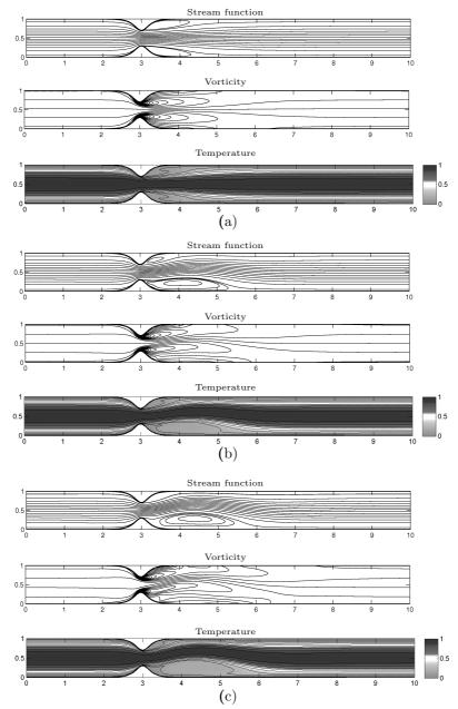
Figure 4.18: Problem 4.6.4: Streamlines, vorticity contours and isotherms 60% stenosis for Re=100, (a)  $Mn_F=Mn_M=0$ , (b)  $Mn_F=82$ ,  $Mn_M=0.025$ , (c)  $Mn_F=164$ ,  $Mn_M=0.1$ .
