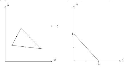
Figure 2.2: Mapping from physical (x, y) plane to the parametric  $(\zeta, \eta)$  plane.
