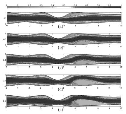
Figure 4.31: Problem 4.6.6: Isotherms for Re = 100: (a)  $Mn_F = 0$ ,  $Mn_M = 0$ , (b)  $Mn_F = 82$ ,  $Mn_M = 0.025$ , (c)  $Mn_F = 164$ ,  $Mn_M = 0.1$ , (d)  $Mn_F = 656$ ,  $Mn_M = 1.2$ , (e)  $Mn_F = 1312$ ,  $Mn_M = 6.4$ .
