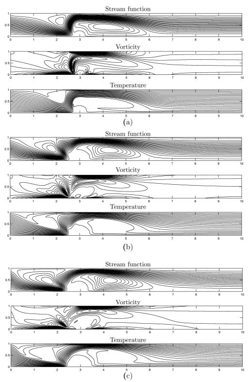
Figure 4.11: Problem 4.6.2: Stream function, vorticity contours and isotherms for (a) Re = 50, Mn = 5250, (b) Re = 20, Mn = 32813, (c) Re = 10, Mn = 131250.
