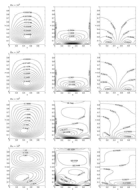
Figure 2.15: Problem 2.4.4.1: Streamlines (L), vorticity contours (M) and isotherms (R) for Ha = 50,  $Ra = 10^3$ ,  $10^4$ ,  $10^5$  and  $10^6$ .
