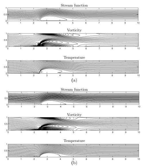
Figure 4.5: Problem 4.6.1: Streamlines, vorticity contours and isotherms for Re = 150, Mn = 115: (a) DRBEM, (b) FEM.
