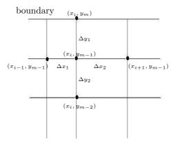
Figure 4.2: Inner nodes for calculation of vorticity boundary conditions.
