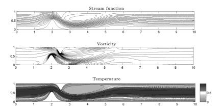
Figure 4.23: Problem 4.6.5: Streamlines, vorticity contours and isotherms, Re = 100,  $Mn_F = 0$ ,  $Mn_M = 0$ .
