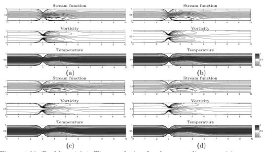
Figure 4.20: Problem 4.6.4: Time evolution for the streamlines, vorticity contours and isotherms, 60% stenosis, for Re=100,  $Mn_F=82$ ,  $Mn_M=0.025$ : (a) t=0.4, (b) t=1.0, (c) t=1.25, (d) t=3.0.
