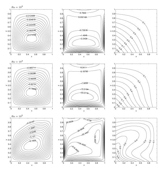
Figure 2.19: Problem 2.4.4.2: Streamlines (L), vorticity contours (M) and isotherms (R) when Ha=30 for  $Ra=10^3$ ,  $10^4$  and  $10^5$ ,  $\phi=0$ ,  $\varphi=0$ .
