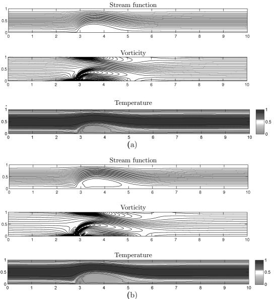
Figure 4.13: Problem 4.6.3 Effects of magnetic field on streamlines, vorticity contours and isotherms for Re = 100 (a)  $Mn_F = 82$ ,  $Mn_M = 0.025$ , (b)  $Mn_F = 164$ ,  $Mn_M = 0.1$ .
