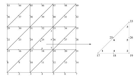
Figure 2.4: Sample discretization of a square region using  $M_e = 18$  elements.
