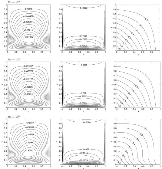
Figure 2.20: Problem 2.4.4.2: Streamlines (L), vorticity contours (M) and isotherms (R) when Ha=80 for  $Ra=10^3$ ,  $10^4$  and  $10^5$ ,  $\phi=0$ ,  $\varphi=0$ .
