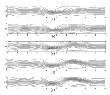
Figure 4.29: Problem 4.6.6: Streamlines for Re = 100: (a)  $Mn_F = 0$ ,  $Mn_M = 0$ , (b)  $Mn_F = 82$ ,  $Mn_M = 0.025$ , (c)  $Mn_F = 164$ ,  $Mn_M = 0.1$ , (d)  $Mn_F = 656$ ,  $Mn_M = 1.2$ , (e)  $Mn_F = 1312$ ,  $Mn_M = 6.4$ .
