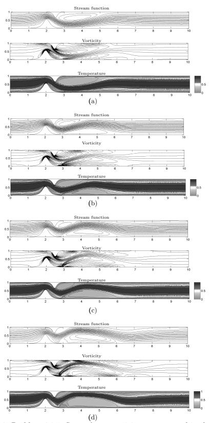
Figure 4.26: Problem 4.6.5: Streamlines, vorticity contours and isotherms, Re = 100, a = 3.0: (a)  $Mn_F = 0$ ,  $Mn_M = 0$ , (b)  $Mn_F = 82$ ,  $Mn_M = 0.025$ , (c)  $Mn_F = 164$ ,  $Mn_M = 0.1$ , (d)  $Mn_F = 656$ ,  $Mn_M = 1.2$ .
