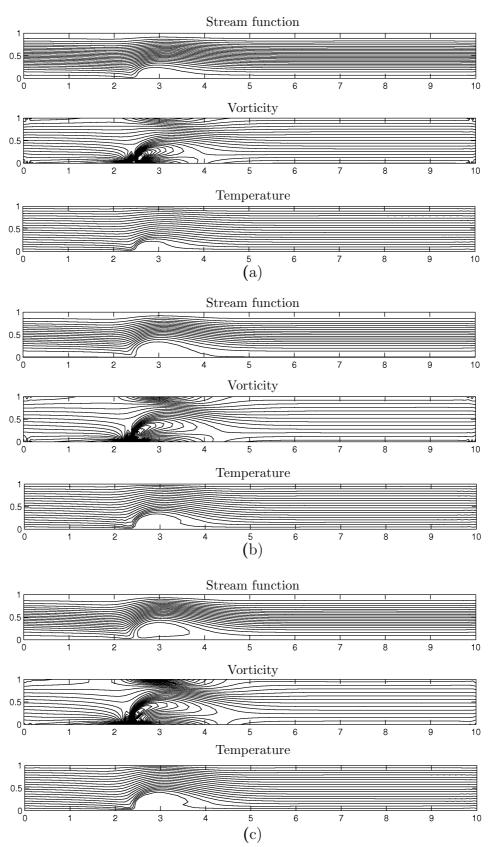
Figure 4.4: Problem 4.6.1: Effects of magnetic field on streamlines, vorticity contours and isotherms (DRBEM) for Re=50,  $(a)\,Mn=115$ ,  $(b)\,Mn=215$ ,  $(c)\,Mn=315$ .
