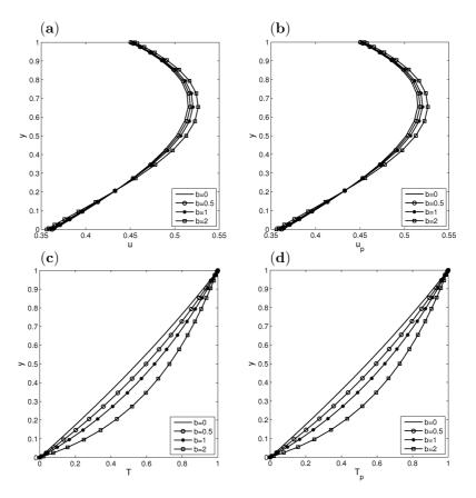
Figure 3.24: Problem 3.4: Steady-state solutions when Ha = 1, a = 1 and  $\beta = 1$  for different thermal conductivity parameter b: (a) u, (b)  $u_p$ , (c) T, (d)  $T_p$ .
