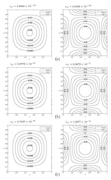
Figure 3.4: Problem 3.2.1: Streamlines (L) and vorticity contours (R) for (a) Re = 0, (b)  $Re = 10^3$ , (c)  $Re = 10^4$ .
