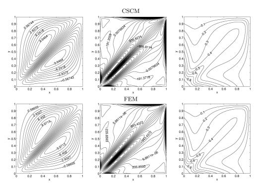
Figure 3.10: Problem 3.2.3: Streamlines (L), vorticity (M) and temperature (R) contours for  $Ra=10^6$  and  $Ha=100, \phi=45, \varphi=45$ .
