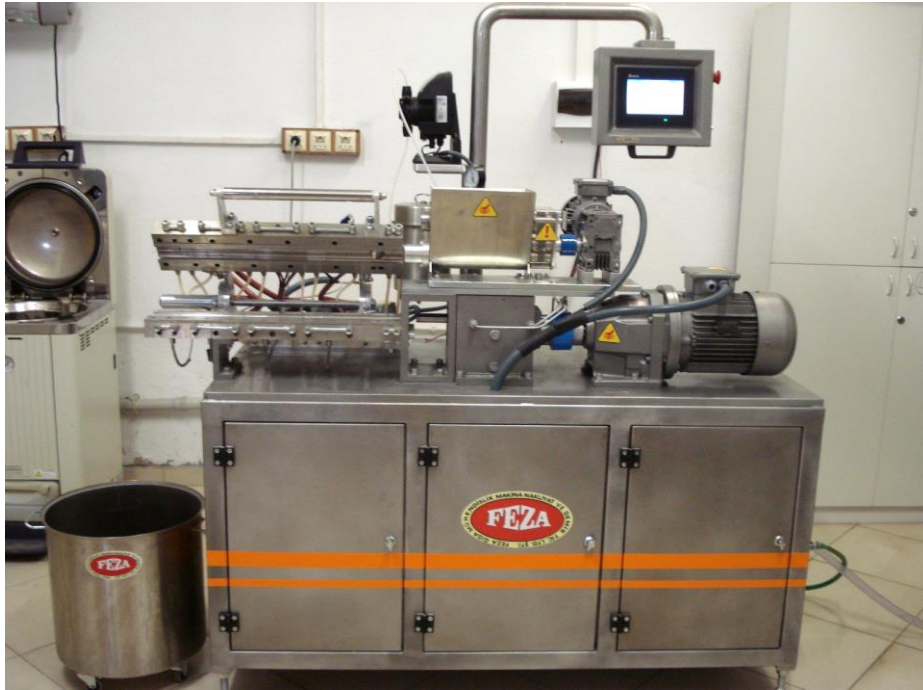
Figure 1. The laboratory scale twin screw extruder used in the study
