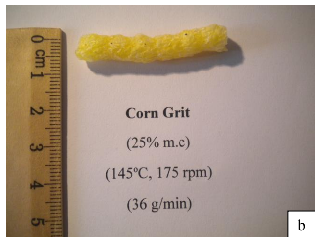
Figure 9. Images of extrudates (25% feed moisture), extruded at 145°C last zone temperature and 175 rpm with feeding rate of 36g/min. a) Red pepper pulp added. b) Control.
