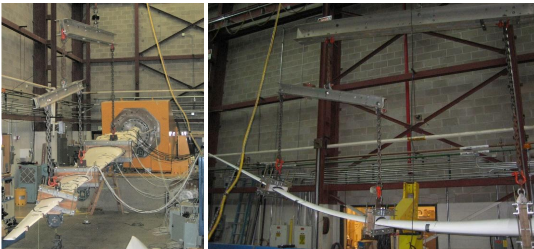
Figure 12: Three-saddle point whiffletree designs used in CX-100 (left) and BSDS (right) blade tests [10]
