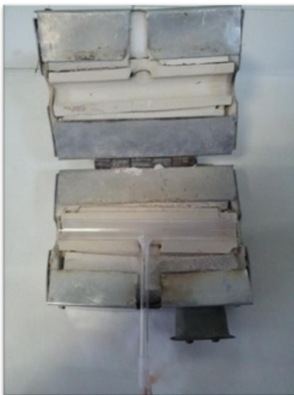
Figure 10: Lab-made ceramic electrical heater used to heat QTA to atomization temperature.
