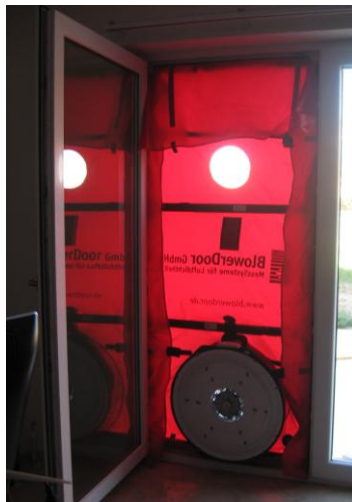
Figure 2.18 Illustration of blower door test
