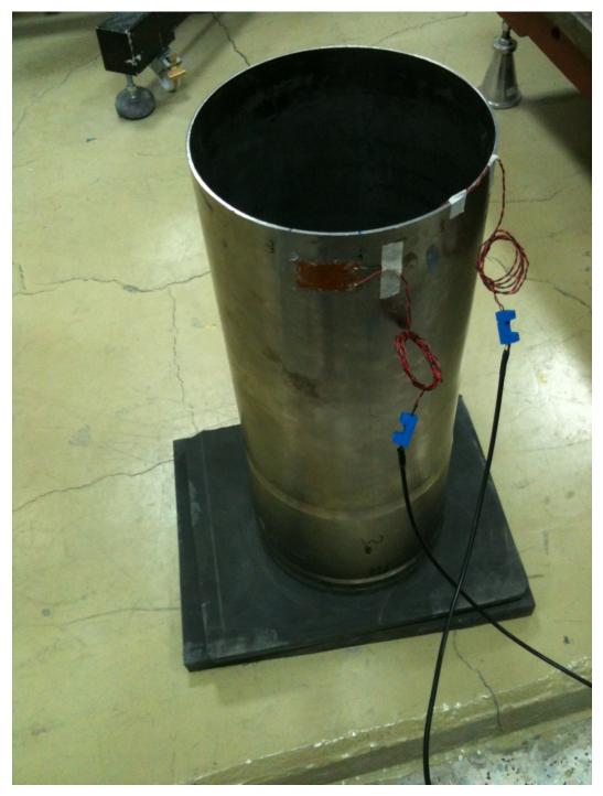
Figure 4-26. Piezoelectric patch on the outer surface of the cylinder
