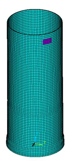
Figure 4-4. Finite element mesh over the 3-D cylinder model
