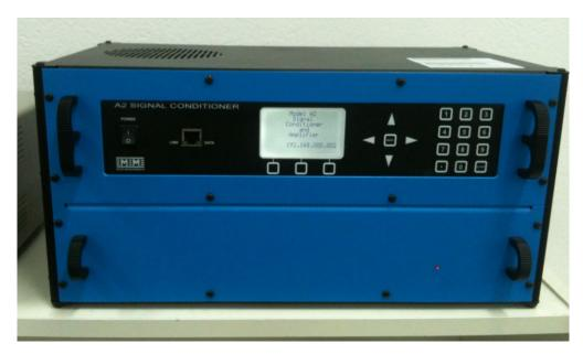
Figure 3-37. Micro Measurement Model A2 Strain gage conditioning unit
