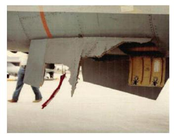
Figure 1-2. Ventral fin failure [9]
