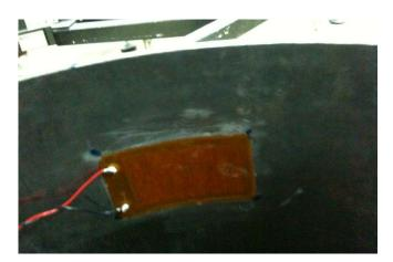
Figure 4-27. Piezoelectric patch on the inner surface of the cylinder
