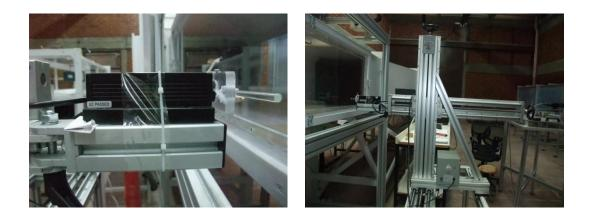
Figure 4.13 Laser System and its Traverse Mechanism
