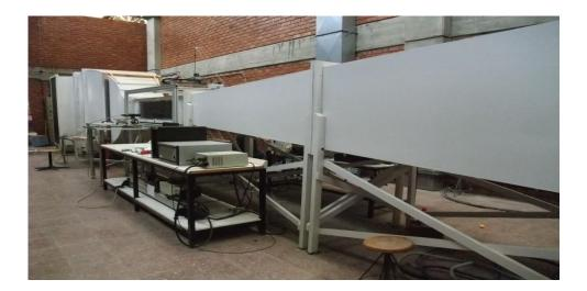
Figure 4.3 Open Loop Low Speed Wind Tunnel
