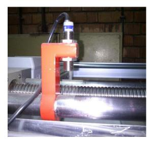
Figure G.4 Sensor of Traverse Mechanism
