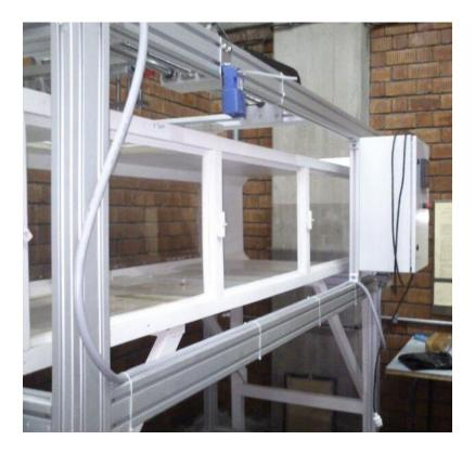
Figure G.6 The Aluminum Structure of Traverse Mechanism
