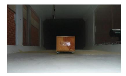
Figure 5.8 Ahmed Body Model Situation in the Test Section
