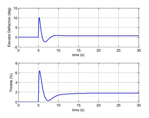
Figure 2.6: Time history of the elevator deflection and throttle of the altitude/velocity acquire control system
