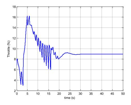
Figure 3.10a: Time history of the throttle, Case 1, SDRE, 50 seconds time scale
