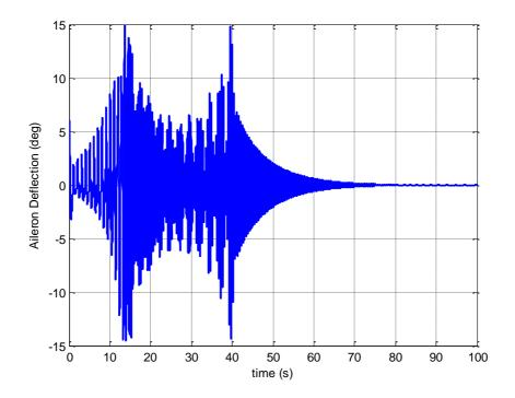
Figure 3.35a: Time history of the aileron deflection, Case 3, SDRE, 100 seconds time scale
