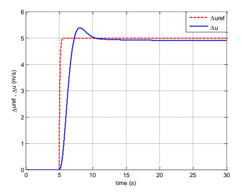
Figure 2.4: Time history of the desired velocity command and velocity output of the altitude/velocity acquire control system
