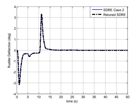
Figure 3.49: Time history of the rudder deflection, SDRE Case 2 vs Retuned SDRE
