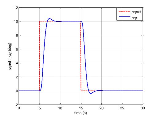
Figure 2.12: Time history of the desired heading command and heading output of the heading acquire control system
