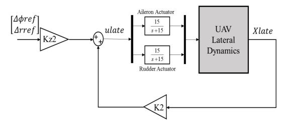
Figure 2.7: Block Diagram for the roll/yaw rate Acquire Control System
