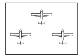
Figure 1.1: V-Formation Geometry
