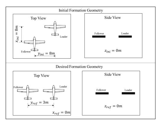
Figure 4.26: Initial and Desired Formation Geometries, Case 3, Lyapunov
