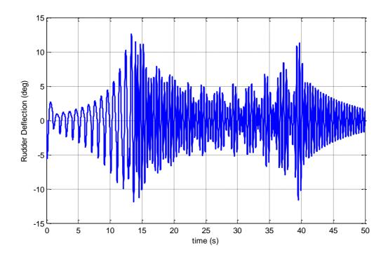
Figure 3.36b: Time history of the rudder deflection, Case 3, SDRE, 50 seconds time scale
