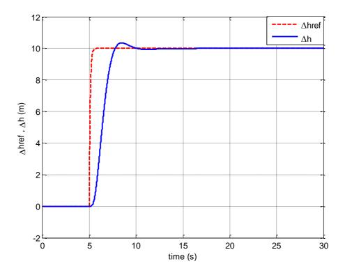
Figure 2.5: Time history of the desired altitude command and altitude output of the altitude/velocity acquire control system
