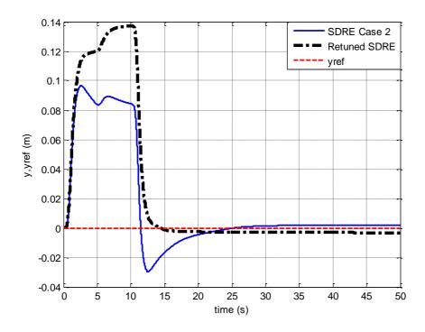
Figure 3.45: Time history of the follower UAV's relative position, y-component, SDRE Case 2 vs Retuned SDRE
