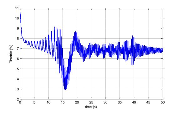
Figure 3.34b: Time history of the throttle, Case 3, SDRE, 50 seconds time scale
