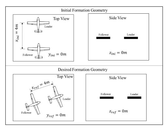
Figure 3.14: Initial and Desired Formation Geometries, Case 2, SDRE
