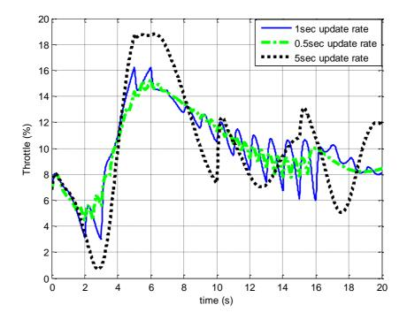
Figure 3.41b: Time history of the throttle with different SDRE update rates, 20 seconds time scale
