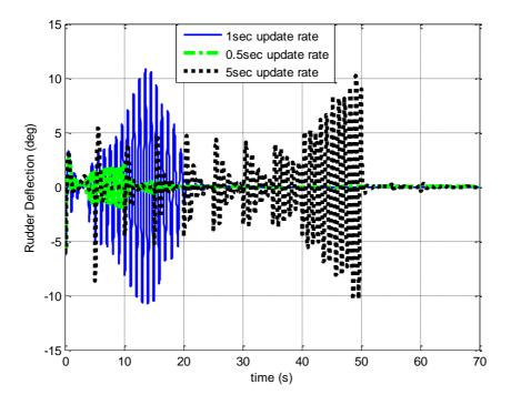
Figure 3.43a: Time history of the rudder deflection with different SDRE update rates, 70 seconds time scale
