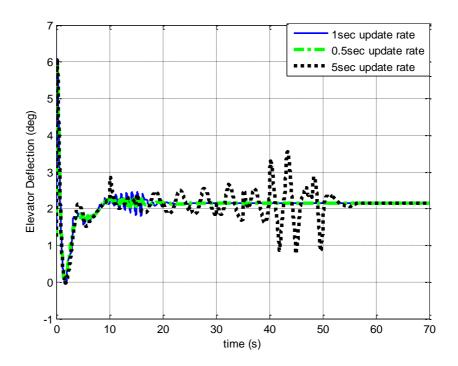
Figure 3.40a: Time history of the elevator deflection with different SDRE update rates, 70 seconds time scale
