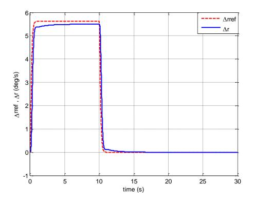
Figure 2.8: Time history of the desired yaw rate command and yaw rate output of the roll/yaw rate acquire control system
