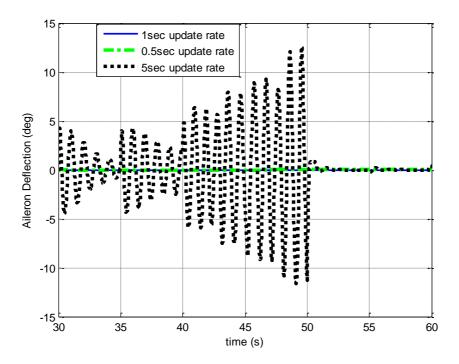
Figure 3.42c: Time history of the aileron deflection with different SDRE update rates, 30-60 seconds time scale
