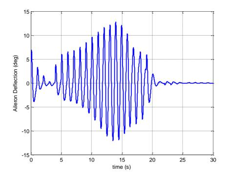
Figure 3.11b: Time history of the aileron deflection, Case 1, SDRE, 30 seconds time scale
