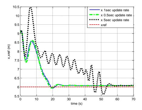
Figure 3.38: Time history of the x-component of the follower UAV's relative position with different SDRE update rates
