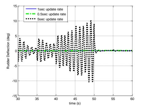
Figure 3.43c: Time history of the rudder deflection with different SDRE update rates, 30-60 seconds time scale
