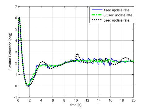
Figure 3.40b: Time history of the elevator deflection with different SDRE update rates, 20 seconds time scale
