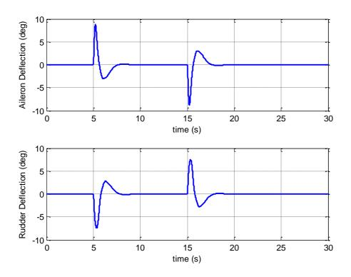
Figure 2.14: Time history of the Aileron and Rudder deflections of the altitude/velocity acquire control system
