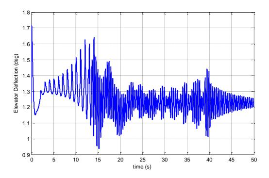
Figure 3.33b: Time history of the elevator deflection, Case 3, SDRE, 50 seconds time scale
