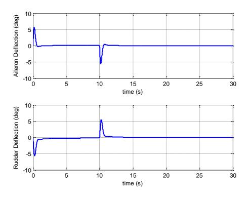
Figure 2.10: Time history of the Aileron and Rudder deflections of the altitude/velocity acquire control system
