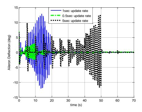
Figure 3.42a: Time history of the aileron deflection with different SDRE update rates, 70 seconds time scale
