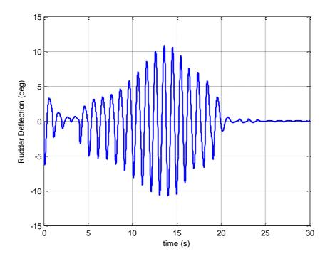
Figure 3.12b: Time history of the rudder deflection, Case 1, SDRE, 30 seconds time scale
