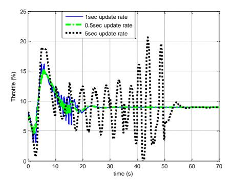
Figure 3.41a: Time history of the throttle with different SDRE update rates, 70 seconds time scale
