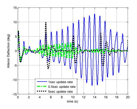
Figure 3.42b: Time history of the aileron deflection with different SDRE update rates, 20 seconds time scale
