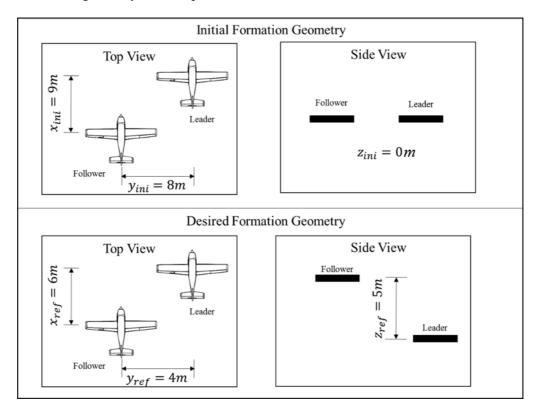
Figure 3.2: Initial and Desired Formation Geometries, Case 1, SDRE
