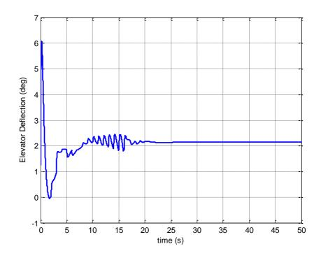
Figure 3.9a: Time history of the elevator deflection, Case 1, SDRE, 50 seconds time scale
