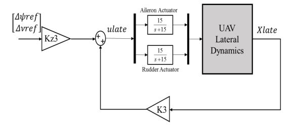
Figure 2.11: Block Diagram for the heading Acquire Control System
