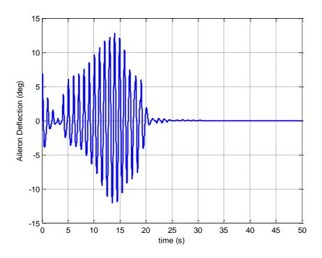
Figure 3.11a: Time history of the aileron deflection, Case 1, SDRE, 50 seconds time scale
