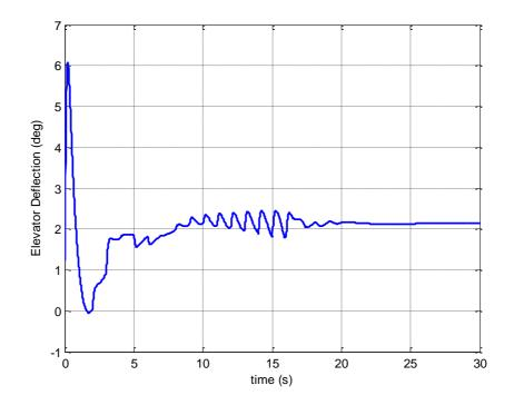
Figure 3.9b: Time history of the elevator deflection, Case 1, SDRE, 30 seconds time scale
