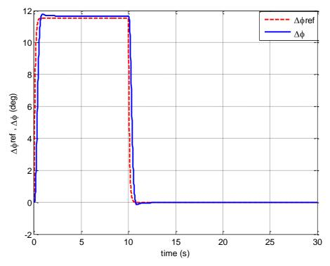
Figure 2.9: Time history of the desired roll command and roll output of the roll/yaw rate acquire control system
