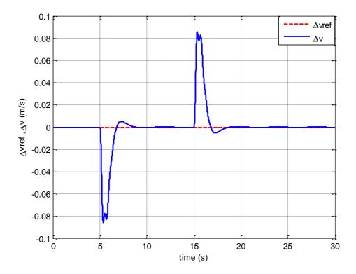
Figure 2.13: Time history of the desired side slip velocity command and side slip velocity output of the heading acquire control system
