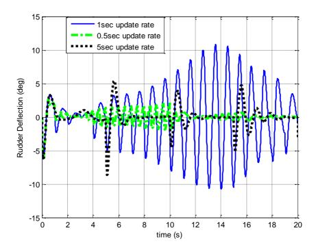
Figure 3.43b: Time history of the rudder deflection with different SDRE update rates, 20 seconds time scale
