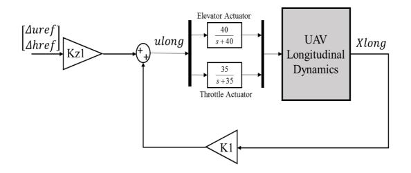
Figure 2.3: Block Diagram for the Altitude/Velocity Acquire Control System
