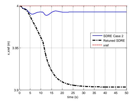
Figure 3.44: Time history of the follower UAV's relative position, x-component, SDRE Case 2 vs Retuned SDRE
