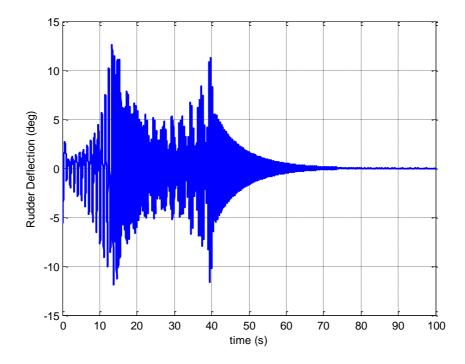
Figure 3.36a: Time history of the rudder deflection, Case 3, SDRE, 100 seconds time scale
