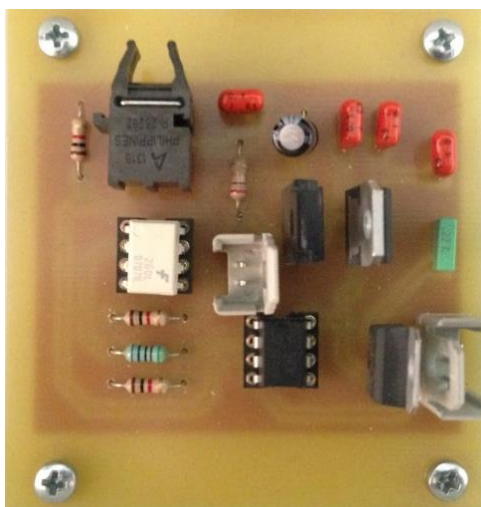
Figure 3.3. The implemented optical triggering system
