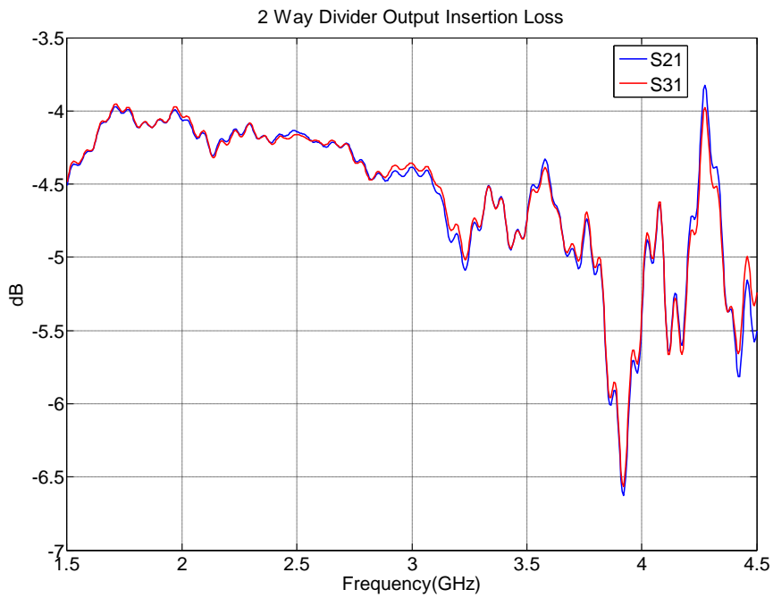
Figure 4.7 Insertion loss characteristics of 2 way divider
