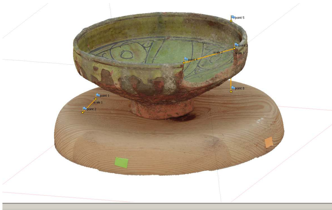
Figure 21: Textured 3D model of the selected ceramic along with digital scale bar and reference measurements.
