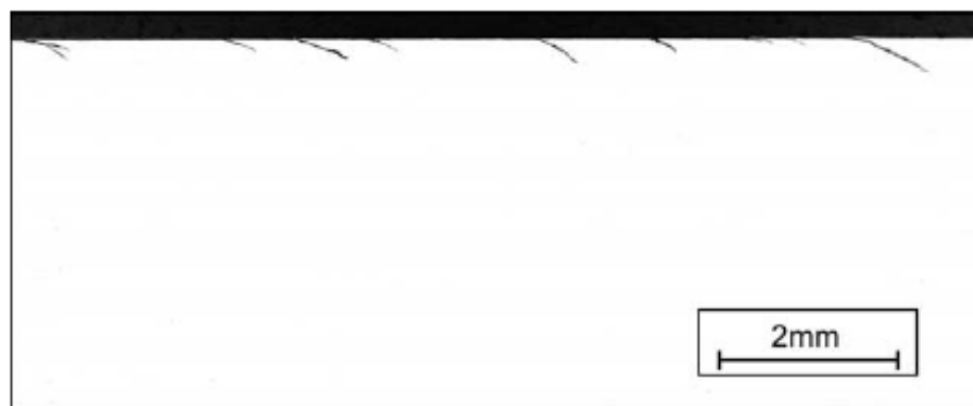
Figure 2.30. Micro graph of rail R350 HT [24].
