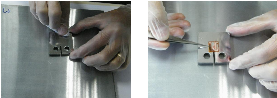
Figure 3.19. Crack foil installation process on the specimen.
