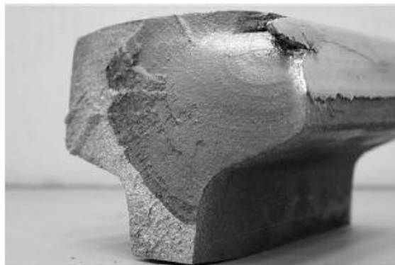
Figure 2.17. Fracture due to head check [16].
