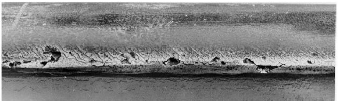
Figure 2.18. Spalling of the rail [16].
