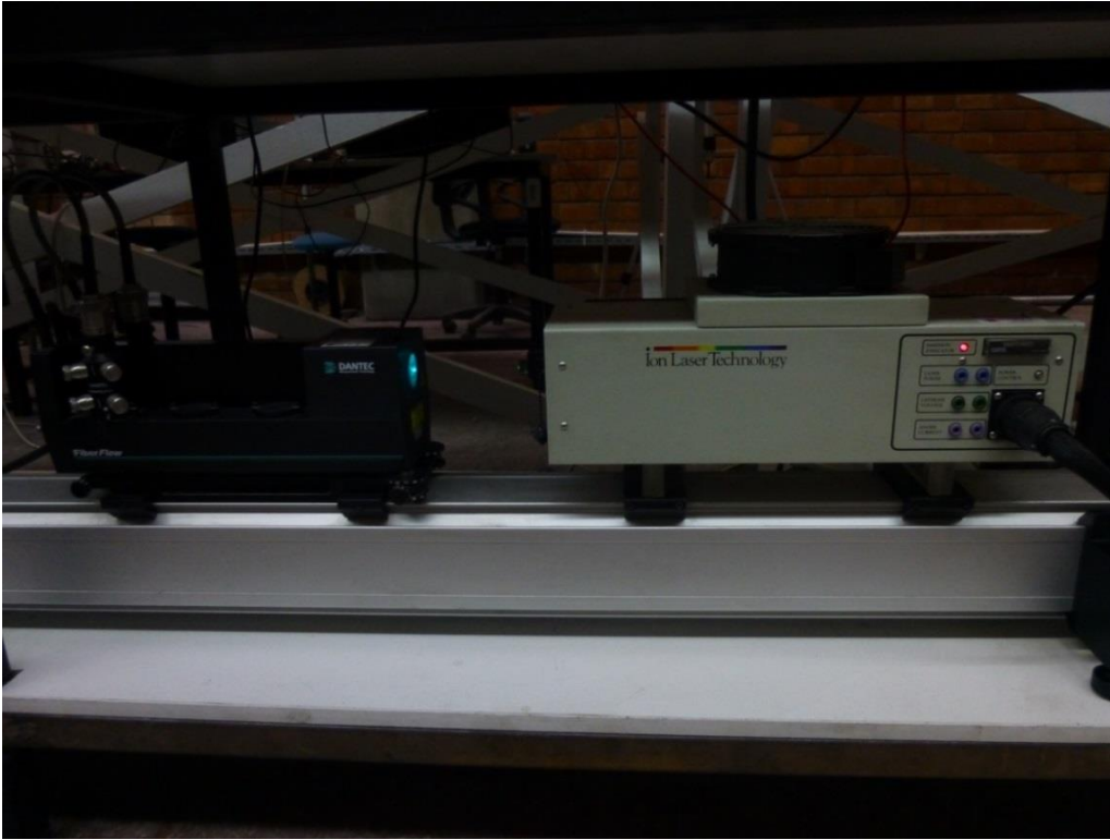
Figure 3.17 The optical and laser units of the LDA system used in the study
