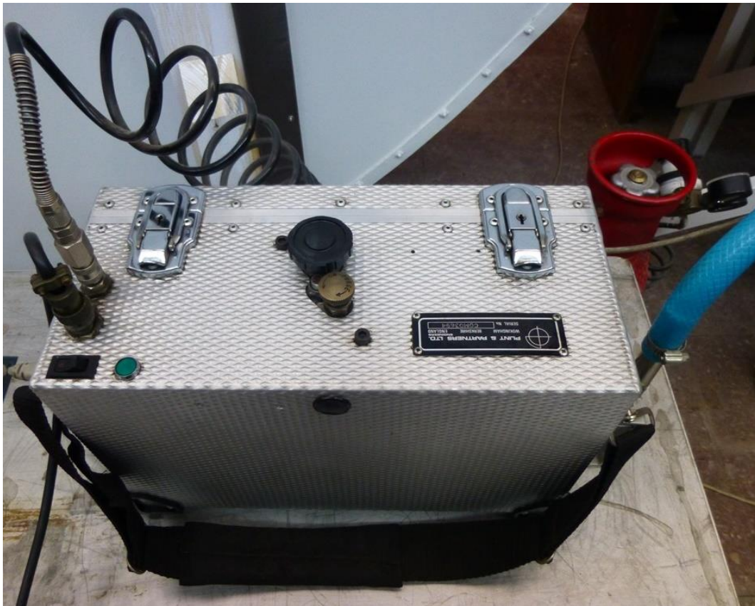
Figure 3.10 The smoke generator used in experiments
