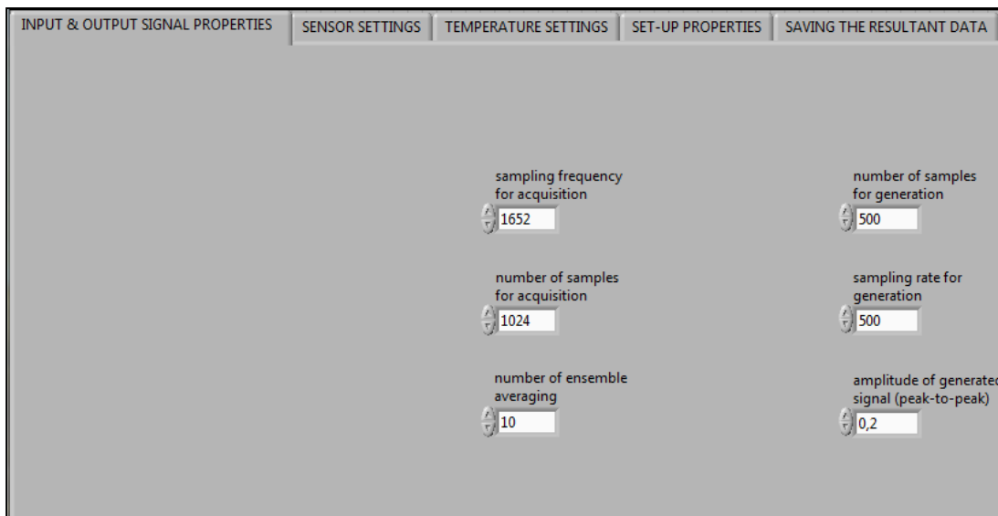
Figure 97. The tab of the user interface for shear specimen testing where the measured and generated signal properties are specified
