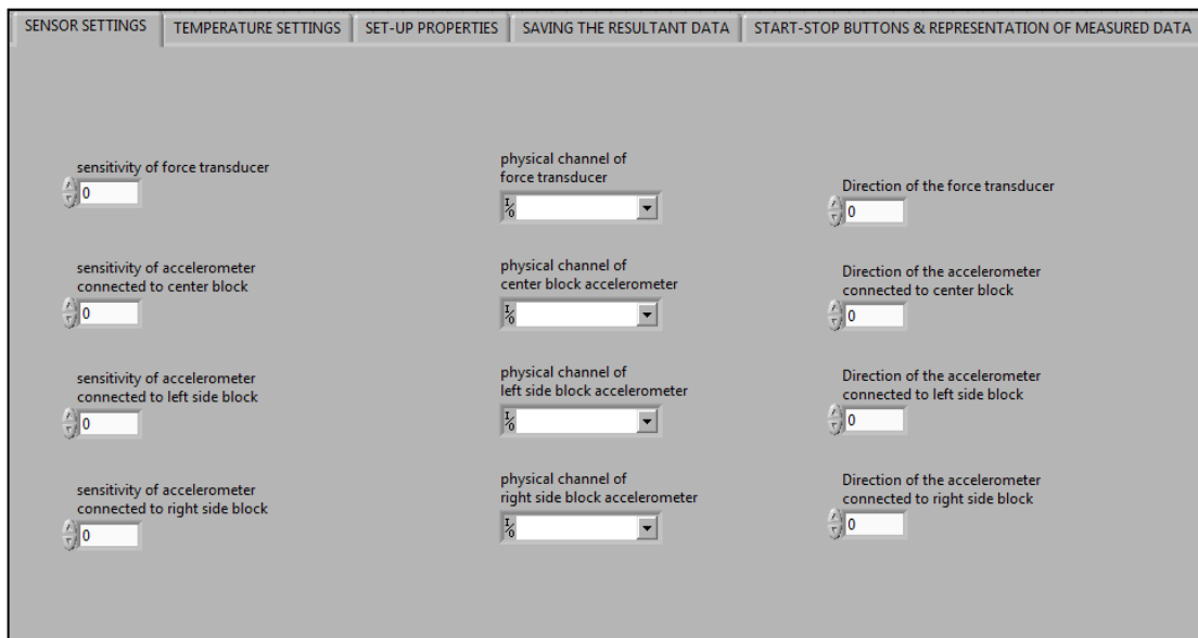
Figure 98. The tab of the user interface for shear specimen testing where the vibration transducer settings are made
