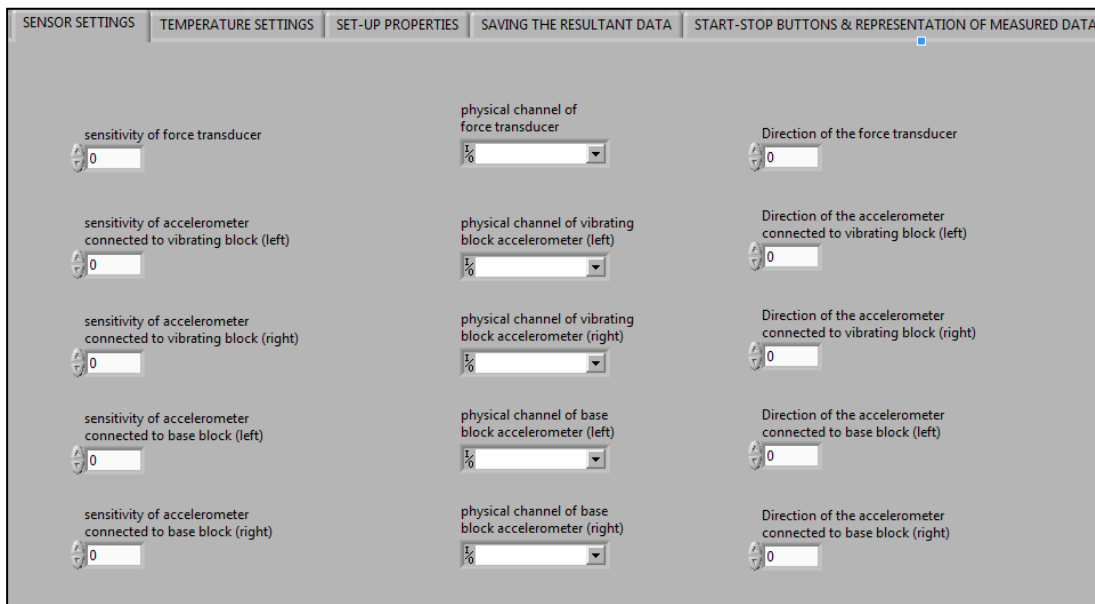
Figure 88. The tab of the user interface for tensile specimen testing where the vibration transducer settings are made
