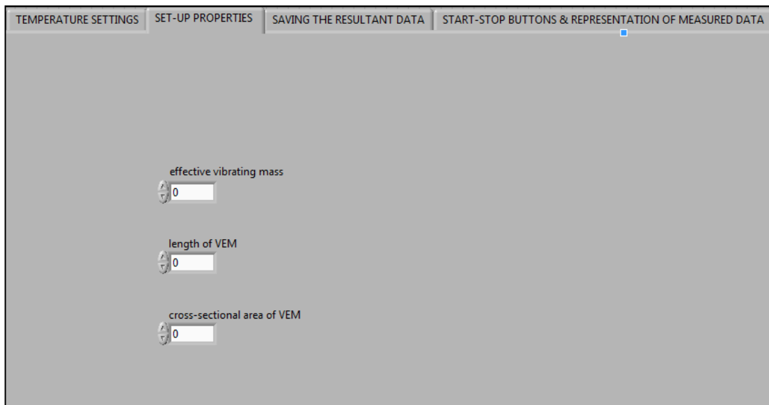
Figure 90. The tab of the user interface for tensile specimen testing where the test set-up properties are specified
