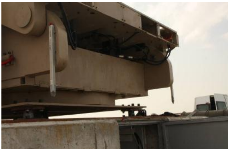
Figure 69. Potentiometer locations on the cradle
