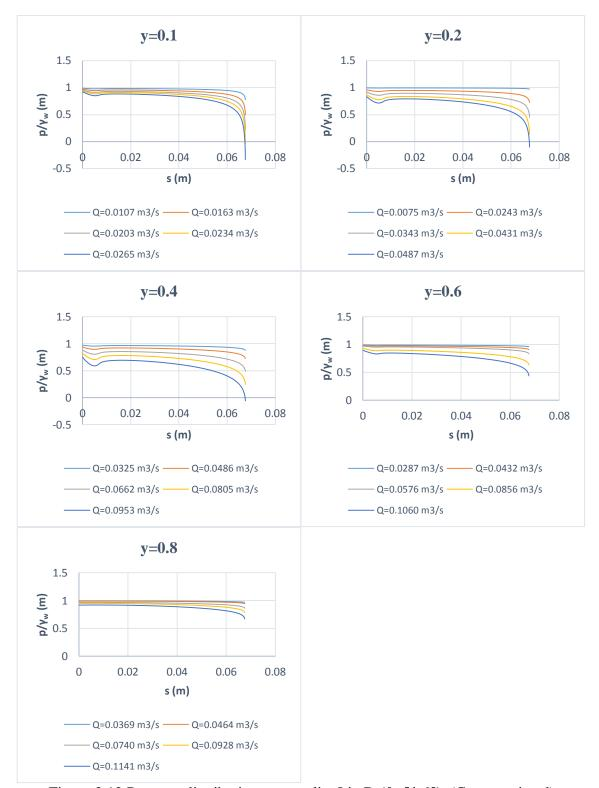
Figure 3.12 Pressure distribution on gate lip, Lip D ( $\theta$ =51.6°). (Computational)
