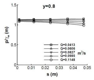
Figure 2.7 Pressure distribution on gate lip, Lip C ( $\theta$ =44.7°). (Aydin et al., 2003)
