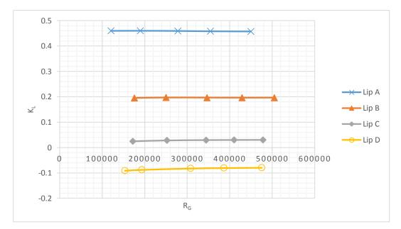
Figure 3.17 Downpull coefficient—Reynolds number relationship, y=0.8 (Computational)
