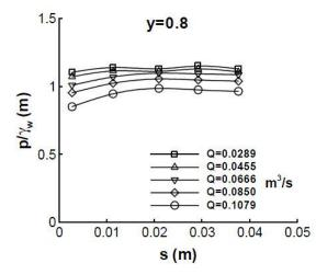
Figure 2.5 Pressure distribution on gate lip, Lip A ( $\theta$ =26.5°). (Aydin et al., 2003)
