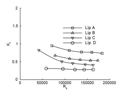
Figure 2.9 Downpull coefficient—Reynolds number relationship, y=0.1 (Aydin et al., 2003)
