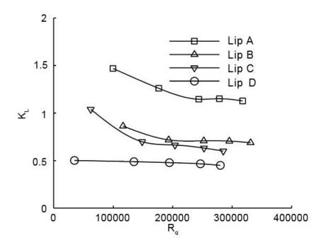
Figure 2.10 Downpull coefficient—Reynolds number relationship, y=0.2 (Aydin et al., 2003)
