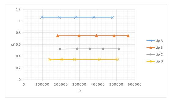
Figure 3.16 Downpull coefficient—Reynolds number relationship, y=0.6 (Computational)
