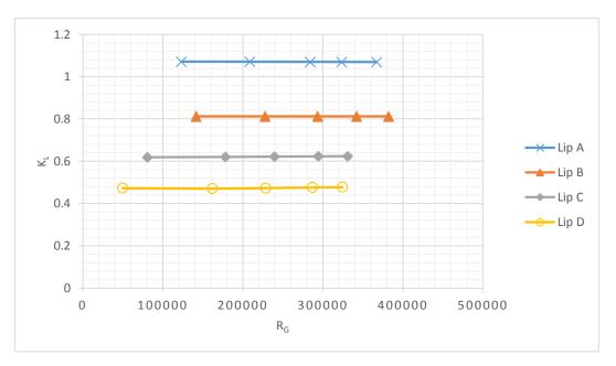
Figure 3.14 Downpull coefficient—Reynolds number relationship, y=0.2 (Computational)
