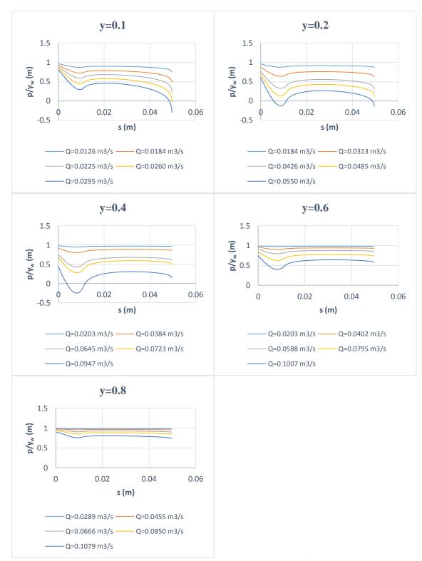
Figure 3.9 Pressure distribution on gate lip, Lip A ( $\theta$ =26.5°). (Computational)
