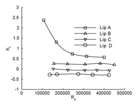
Figure 2.13 Downpull coefficient—Reynolds number relationship, y=0.8 (Aydin et al., 2003)
