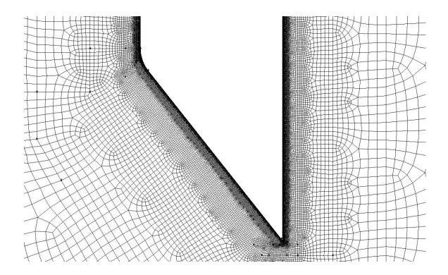
Figure 3.4 Mesh around the gate
