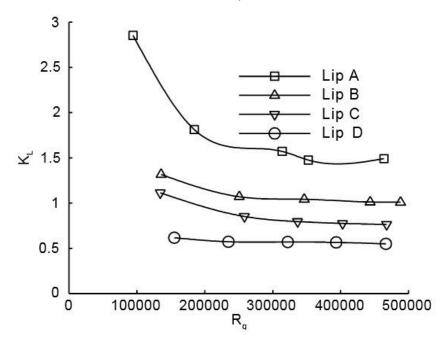
Figure 2.11 Downpull coefficient—Reynolds number relationship, y=0.4 (Aydin et al., 2003)
