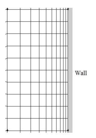
Figure 3.6 Near-wall mesh
