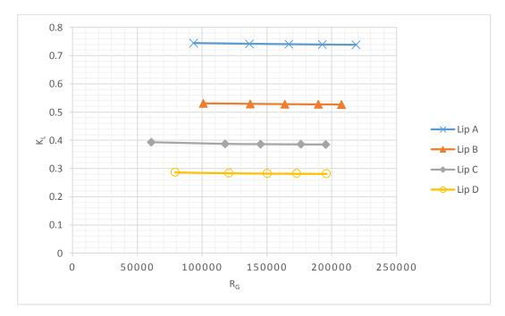
Figure 3.13 Downpull coefficient—Reynolds number relationship, y=0.1 (Computational)
