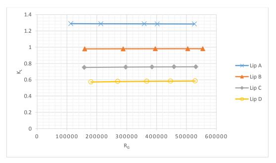
Figure 3.15 Downpull coefficient—Reynolds number relationship, y=0.4 (Computational)
