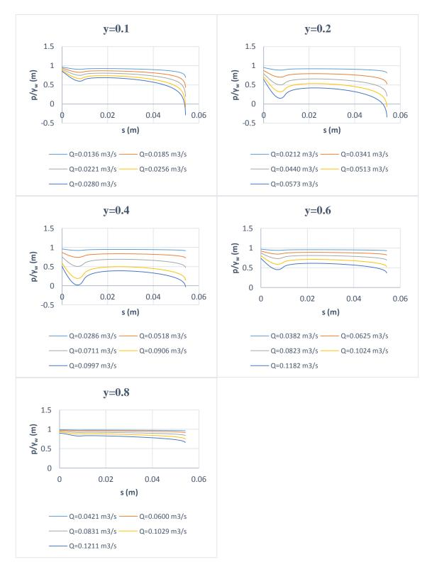
Figure 3.10 Pressure distribution on gate lip, Lip B ( $\theta$ =36.7°). (Computational)
