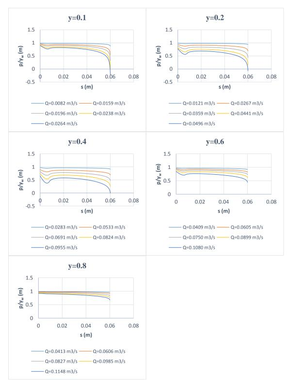
Figure 3.11 Pressure distribution on gate lip, Lip C ( $\theta$ =44.7°). (Computational)
