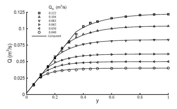
Figure 3.8 Maximum system discharge (Aydin et al., 2003)
