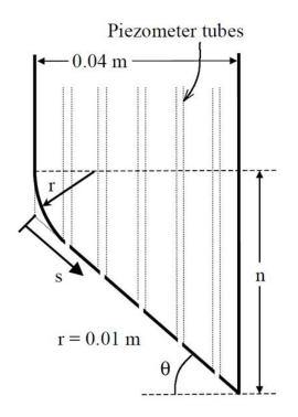
Figure 2.4 Gate lip details (Aydin et al., 2003)
