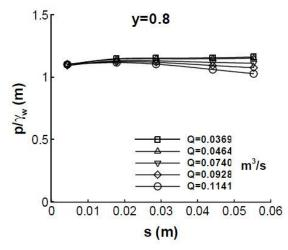
Figure 2.8 Pressure distribution on gate lip, Lip D ( $\theta$ =51.6°). (Aydin et al., 2003)
