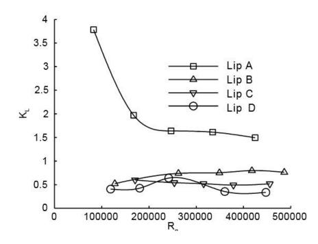
Figure 2.12 Downpull coefficient—Reynolds number relationship, y=0.6 (Aydin et al., 2003)
