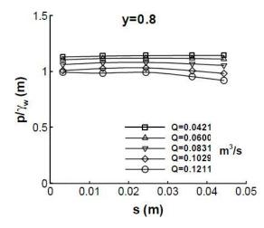
Figure 2.6 Pressure distribution on gate lip, Lip B ( $\theta$ =36.7°). (Aydin et al., 2003)
