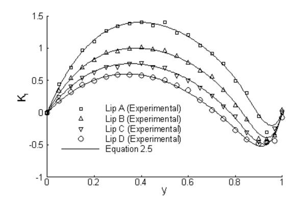
Figure 2.14 Downpull coefficient as a function of gate opening and gate lip angle (Aydin et al., 2003)
