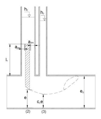
Figure 2.3 Details of gate region (Aydin et al., 2003)
