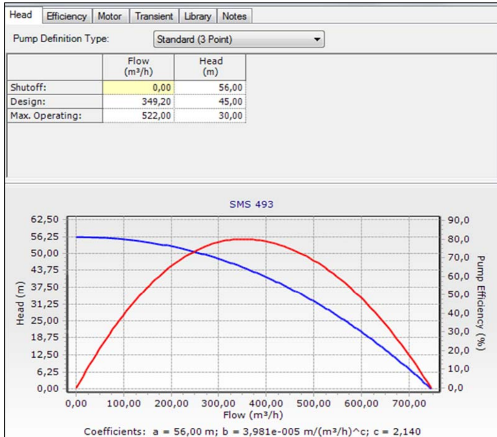
Figure 5.5: Pump Curve of SMS (Pump 3)
