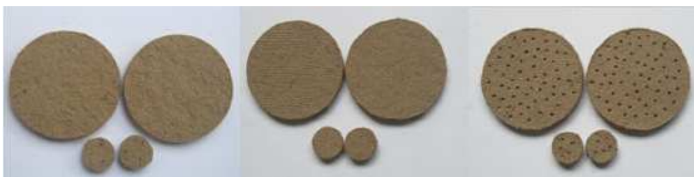
Figure 2.27 A set of specimens with various finishing; rough surface (left), screen surface (middle) and perforated surface (right) (Sihabut & Laemsak, 2012)
