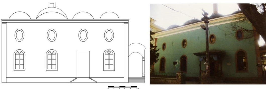
Figure. 154 The drawing and photograph of north facade of Söğüt Çelebi Mehmet Mosque. Source: Drawing by the author based on the information in VGM Archive. Photograph: Author 2011.
