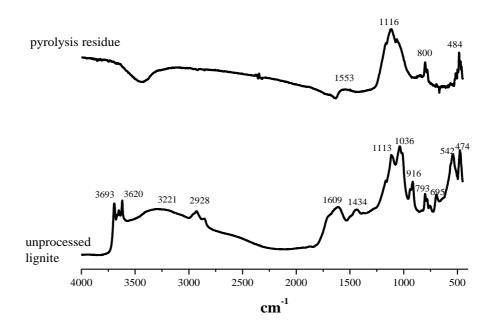
Figure 5.3. DRIFT spectra of coal and its pyrolysis residue.
