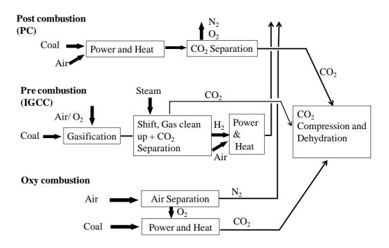
Figure 6.1. Three technologies for  $CO_2$  capture from fossil fuels (GCCSI, 2012).
