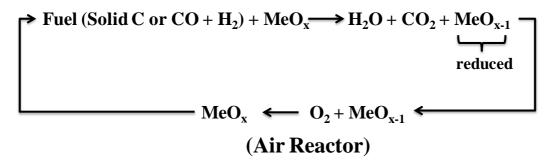
Figure 6.2. Chemical looping combustion system.
