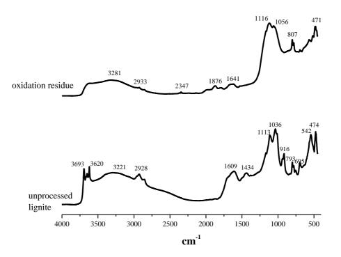
Figure 5.8. DRIFTS spectra of unprocessed lignite and its oxidation residue.
