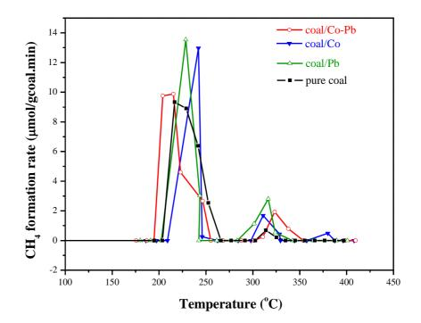
Figure 6.18. CH<sub>4</sub> formation rates under air flow using the constant coal: metal oxide ratio of 10 (wt:wt).
