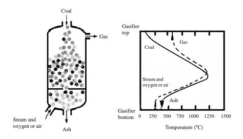
Figure 2.3. Fixed-bed gasifier (van Dyk et al., 2006).
