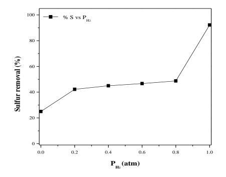
Figure 5.10. Sulfur removal percentages of Tuncbilek lignite vs. hydrogen partial pressure.
