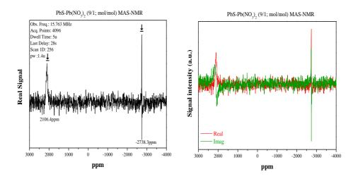
Figure 6.11. The <sup>207</sup>Pb MAS spectrum of reference compounds of PbS-Pb(NO<sub>3</sub>)<sub>2</sub>.
