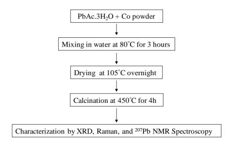
Figure 6.3. Co-Pb metal oxide preparation steps.
