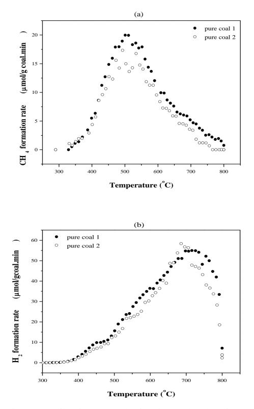
Figure 5.1. CH<sub>4</sub> formation rates (a) and H<sub>2</sub> formation rates (b) under N<sub>2</sub> flow.
