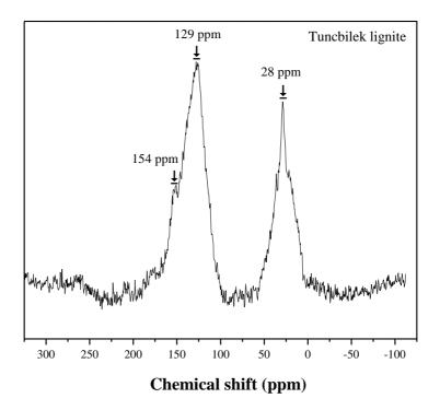
Figure 4.6. Carbon NMR spectrum of Tuncbilek lignite.
