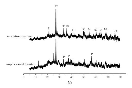
Figure 5.7. XRD patterns of unprocessed lignite and its oxidation residue.
