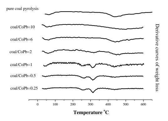
Figure 6.7. TGA pyrolysis thermograms of coal in the presence of different metal oxide contents.
