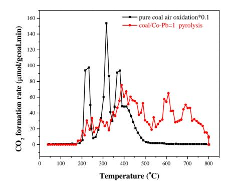
Figure 6.17.  $CO_2$  formation rates of pure coal during air oxidation and coal/Co-Pb =1during pyrolysis.
