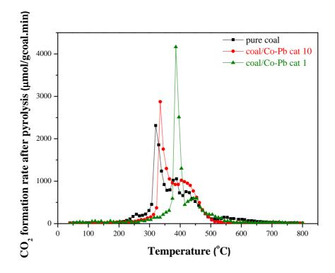
Figure 6.21. CO<sub>2</sub> emission during air oxidation of the pyrolysis residues.
