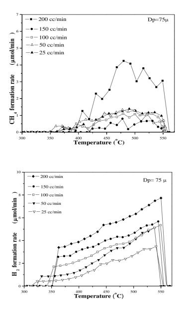
Figure B.2. (a)  $CH_4$  and (b)  $H_2$  formation rates under non-isothermal condition and different flow rates.
