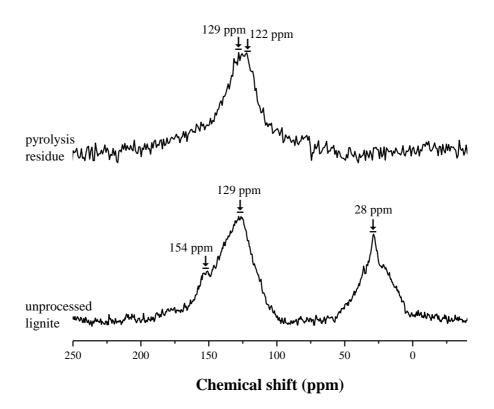
Figure 5.5. Aliphatic, aromatic and C=O double bond traces of unprocessed lignite and lignite residue after pyrolysis.
