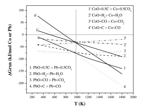
Figure 6.6. Comparison between the PbO and CoO reduction with Carbon, Hydrogen, and Carbon monoxide.
