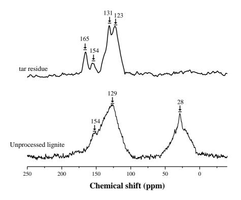
Figure 5.17. <sup>13</sup>C NMR spectra of the unprocessed lignite and hydrogenated liquid coal residue.
