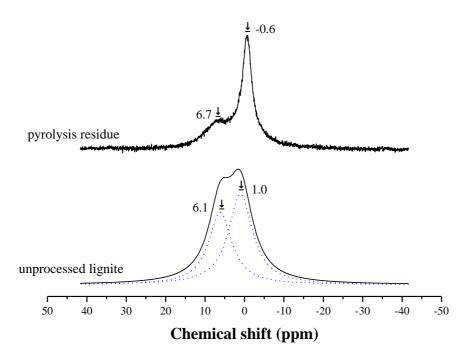
Figure 5.4. <sup>1</sup>H NMR spectra of unprocessed lignite and its pyrolysis residue.
