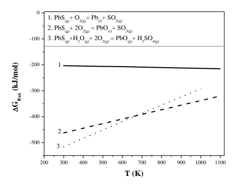
Figure 6.24. Oxidation thermodynamics of PbS.
