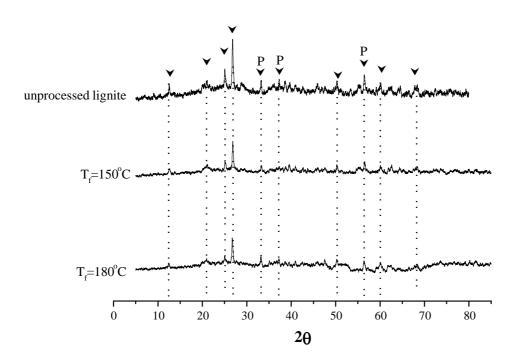
Figure 5.23. Inorganic structure of lignite residue after wet air oxidation at 150°C and 180°C.
