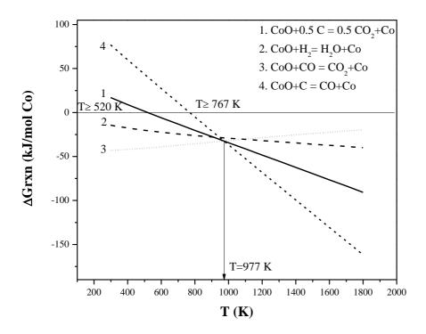
Figure 6.5. Standard Gibbs free energy change during Cobalt oxide reduction.
