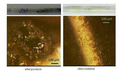
Figure 6.22. The visual and microscopic images of PbO reduction to metallic Pb during pyrolysis and oxidation reactions.
