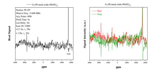
Figure 6.13. The <sup>207</sup>Pb MAS spectrum of Co-Pb metal oxide- Pb(NO<sub>3</sub>)<sub>2</sub> with spin-echo.
