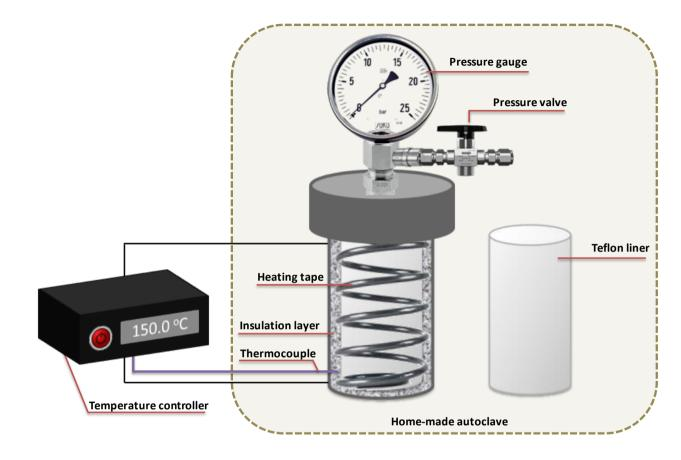
Figure 3.3. Schematic representation of experimental set up for oxy-desulfurization reaction tests.
