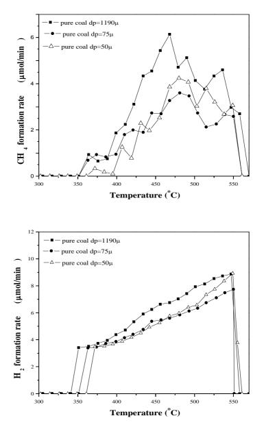
Figure B.1. Pore diffusion effects on  $CH_4$  (a) and  $H_2$  (b) formation rates for different particle sizes.
