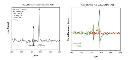
Figure 6.12. The <sup>207</sup>Pb MAS spectrum of reference compounds of PbSO<sub>4</sub>-Pb(NO<sub>3</sub>)<sub>2</sub>.
