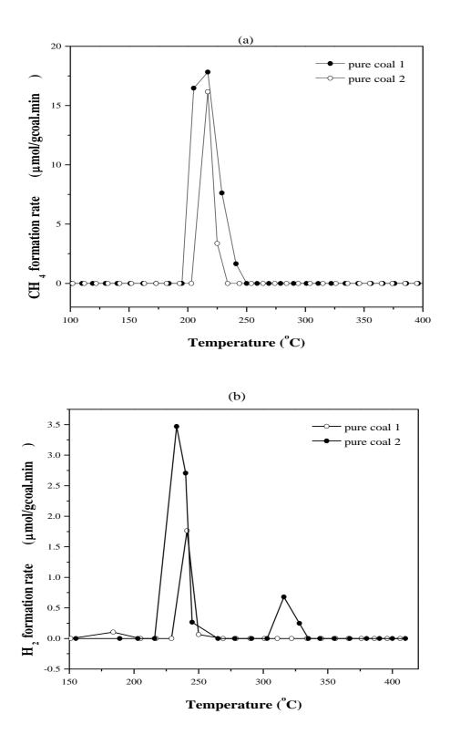
Figure 5.6.  $CH_4$  formation rates (a) and  $H_2$  formation rates (b) under air flow.
