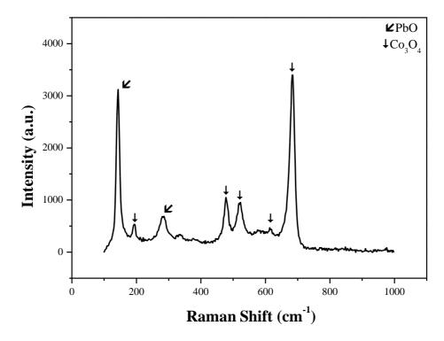
Figure 6.9. Raman spectra of Co-Pb metal oxide.
