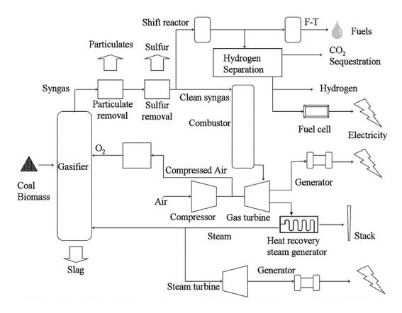
Figure 1.1. Schematic diagram of coal gasification processes for electricity, hydrogen, liquid fuel production (Fan et al., 2008).
