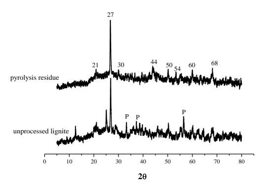
Figure 5.2. XRD pattern of unprocessed lignite and its pyrolysis residue.
