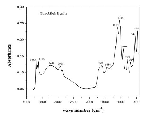
Figure 4.4. DRIFT spectrum of Tuncbilek lignite.
