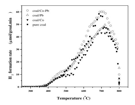
Figure 6.15.  $H_2$  formation rates under  $N_2$  flow using the constant coal: metal oxide ratio of 10 (wt/wt).
