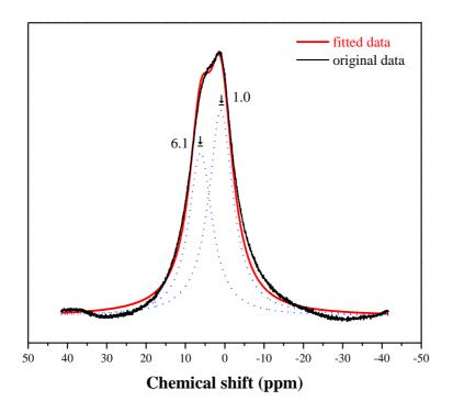
Figure 4.5. Proton NMR spectrum of Tuncbilek lignite.
