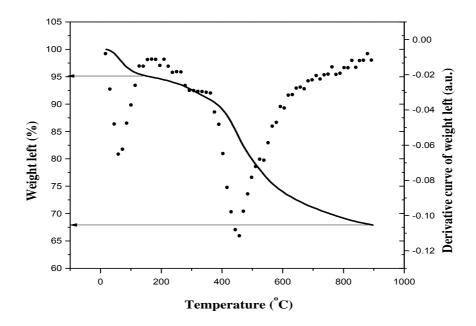
Figure 4.1. TGA and DTG curves of coal sample under  $N_2$  flow. Solid line represents the TGA, while dotted line represents the DTG.
