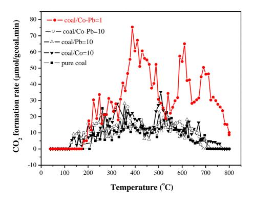
Figure 6.16.  $CO_2$  formation rates under  $N_2$  flow in the presence and absence of metal oxide.
