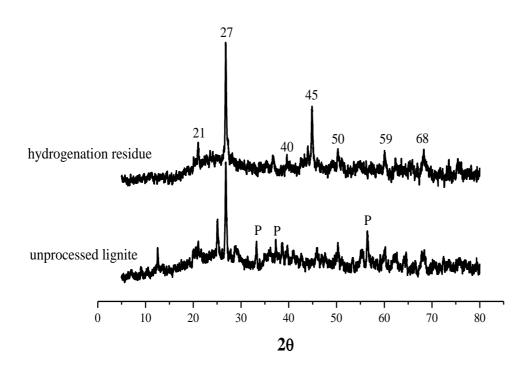
Figure 5.11. X-ray patterns of unprocessed lignite and its hydrogenation residue.
