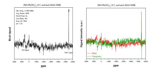
Figure 6.10. The <sup>207</sup>Pb MAS spectrum of reference compounds of PbO-Pb(NO<sub>3</sub>)<sub>2</sub>.
