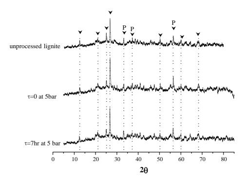
Figure 5.21. Inorganic structure of lignite residue after wet air oxidation for the longest and shortest duration.
