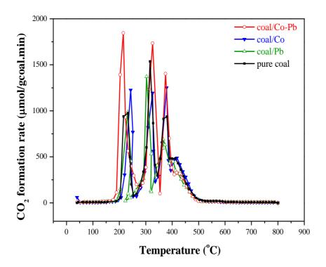
Figure 6.20. CO<sub>2</sub> formation rate in the presence and absence of metal oxides using the fix coal: metal oxide ratio of 10.
