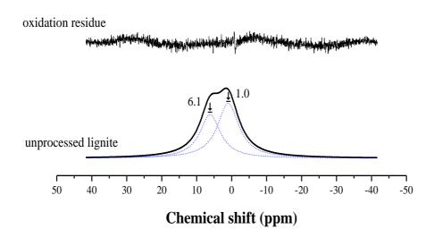
Figure 5.9. <sup>1</sup>H NMR spectra of unprocessed lignite and its oxidation residue.
