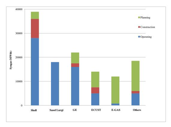
Figure 2.2. Technology distribution of gasification (NETL, 2010).
