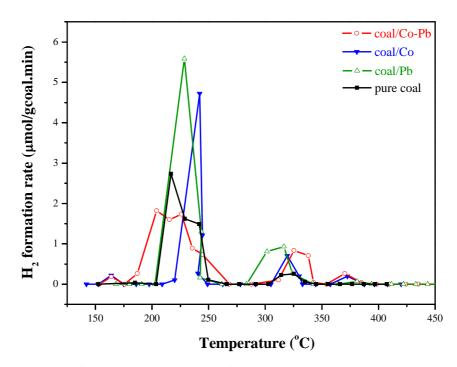
Figure 6.19.  $H_2$  formation rates under air flow using the constant coal: metal oxide ratio of 10 (wt:wt).
