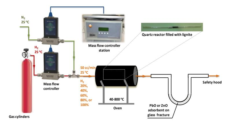
Figure 3.2. Schematic representation of experimental set up for hydrogenation reaction tests.
