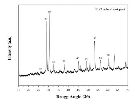
Figure 5.12. XRD pattern of commercial PbO after hydrogenation experiment
