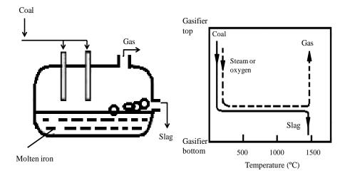
Figure 2.6. Molten-bed gasifier (Kabe et al., 2004a).
