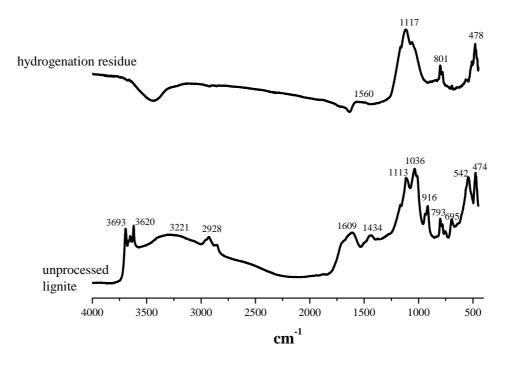
Figure 5.14. DRIFT spectra of unprocessed lignite and its hydrogenation residue.
