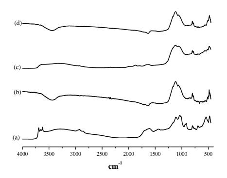
Figure 5.19. DRIFT spectra of (a) coal samples, (b) coal sample residue after pyrolysis, (c) coal sample residue after oxidation, (d) coal sample residue after hydrogenation Tuncbilek lignite.
