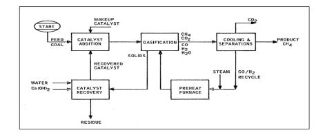
Figure 2.9. Exxon Catalytic Coal Gasification Process flowchart (Nahas, 1983).
