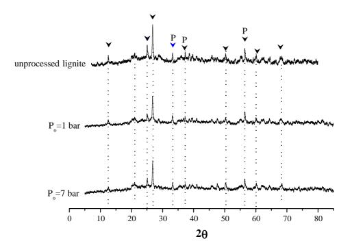
Figure 5.22. Inorganic structure of lignite residue after wet air oxidation at 1 bar and 7 bar.
