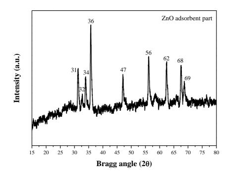
Figure 5.13. XRD pattern of commercial ZnO after hydrogenation experiment.
