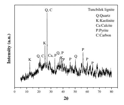
Figure 4.3. XRD pattern of Tuncbilek lignite.
