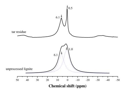
Figure 5.16. <sup>1</sup>H NMR spectra of the unprocessed lignite and hydrogenated liquid coal residue.
