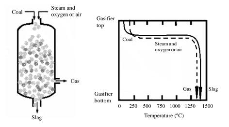
Figure 2.5. Entrained-bed gasifier (Kabe et al., 2004a).
