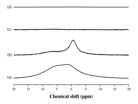
Figure 5.20. <sup>1</sup>H MAS NMR spectra of (a) coal samples, (b) coal sample residue after pyrolysis, (c) coal sample residue after oxidation, (d) coal sample residue after hydrogenation Tuncbilek lignite.
