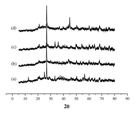
Figure 5.18. XRD patterns of (a) unprocessed lignite, (b) coal sample residue after pyrolysis, (c) coal sample residue after oxidation, (d) coal sample residue after hydrogenation Tuncbilek lignite.
