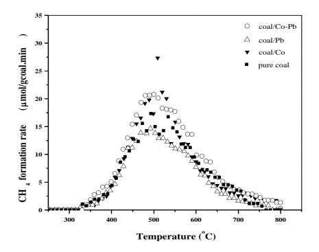
Figure 6.14. CH<sub>4</sub> formation rates under  $N_2$  flow using the constant coal: metal oxide ratio of 10 (wt/wt).
