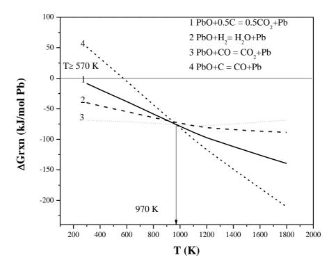
Figure 6.4. Standard Gibbs free energy change during lead oxide reduction.
