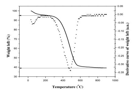
Figure 4.2. TGA and DTG curves of coal sample under air flow. Solid line represents the TGA, while dotted line represents the DTG.
