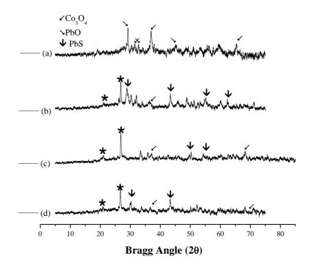
Figure 6.23. In-situ sulfur capture potential of PbO: (a) fresh Co-Pb metal oxide, (b) after pyrolysis, (c) after oxidation, and (d) after hydrogenation.
