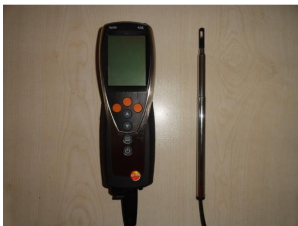
Figure 4.18: Hot wire probe and multifunction measuring instrument
