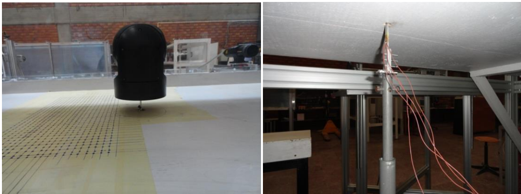
Figure 4.14: Loadcell-model assembly in test section
