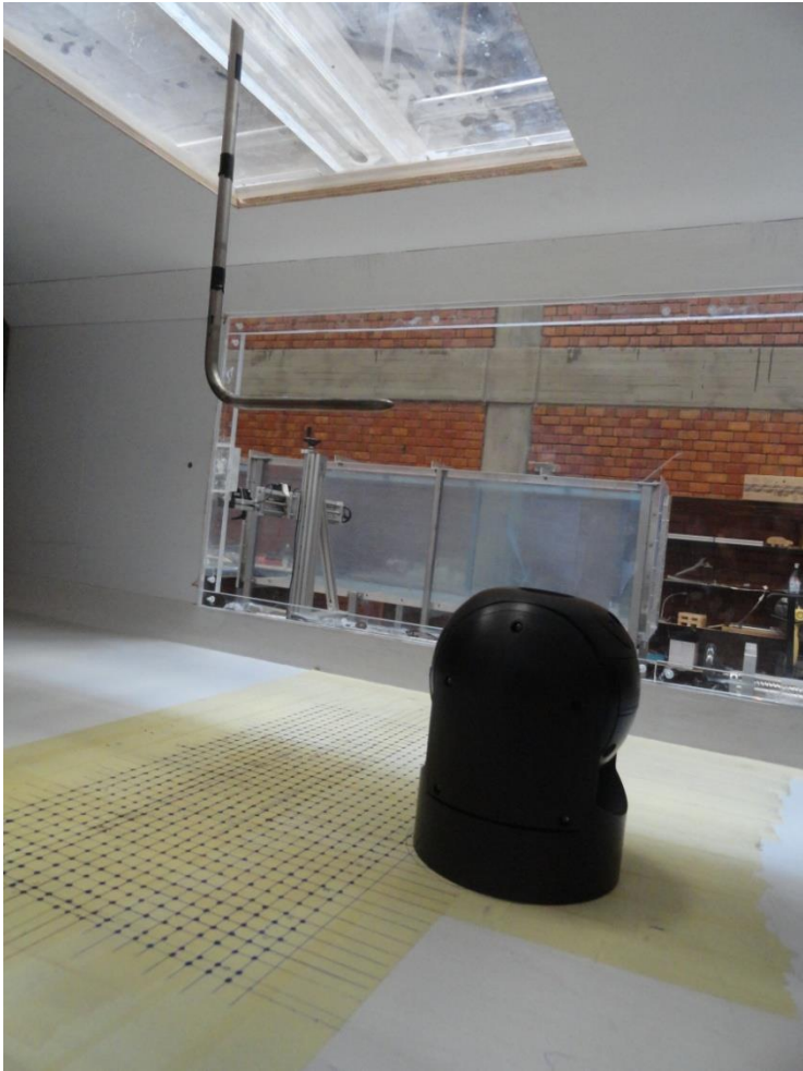
Figure 4.15: Pitot-static tube in test section
