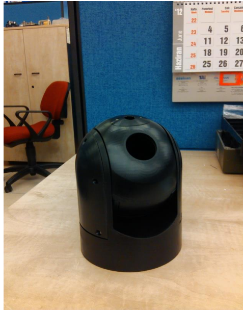
Figure 1.4: Prototype of the mini gimbal
