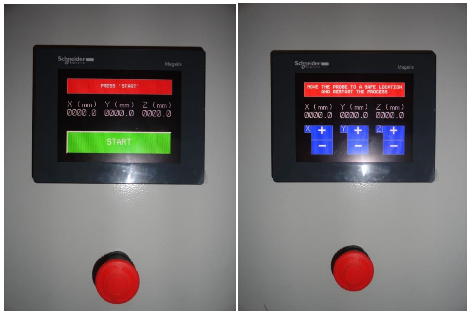
Figure 4.8: Touch-operated control panel of the traverse mechanism
