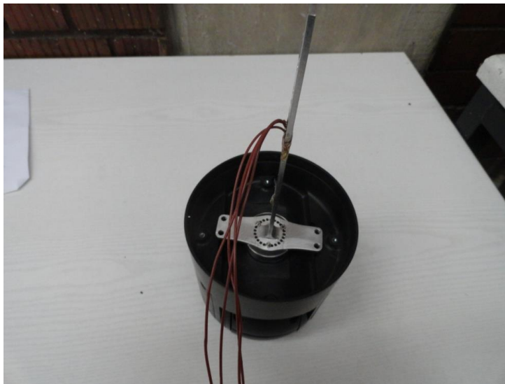
Figure 4.12: Assembly of the load-cell and the model
