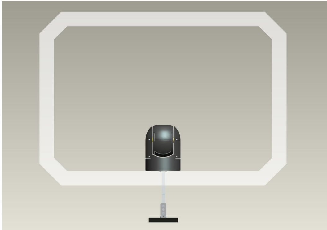
Figure A.16: Assembly of the gimbal and the load-cell (balance) in the wind tunnel
