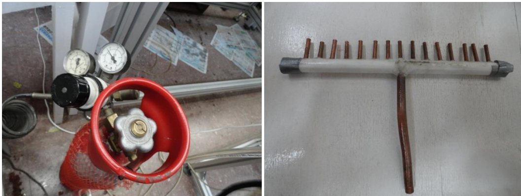
Figure 4.19: CO 2 smoke generator tube and comb-like instrument
