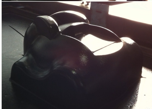
Figure 4.2: Vacuum Forming Stages of the Outer Cover
