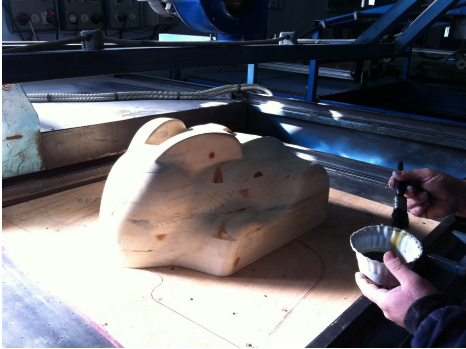
Figure 4.1: Wooden Mold of the Outer Cover
