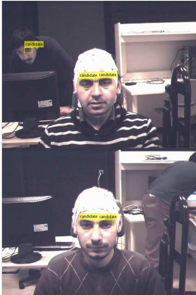
Figure 3.9: Some examples of right eye region candidates found for subjects A, B,C and D respectively
