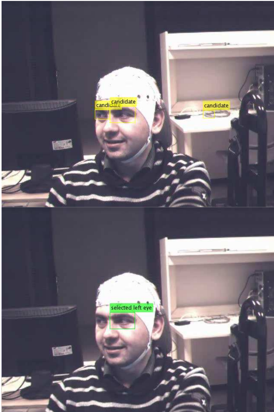
Figure 3.22: An example of valid left eye region selection among candidates for subject A
