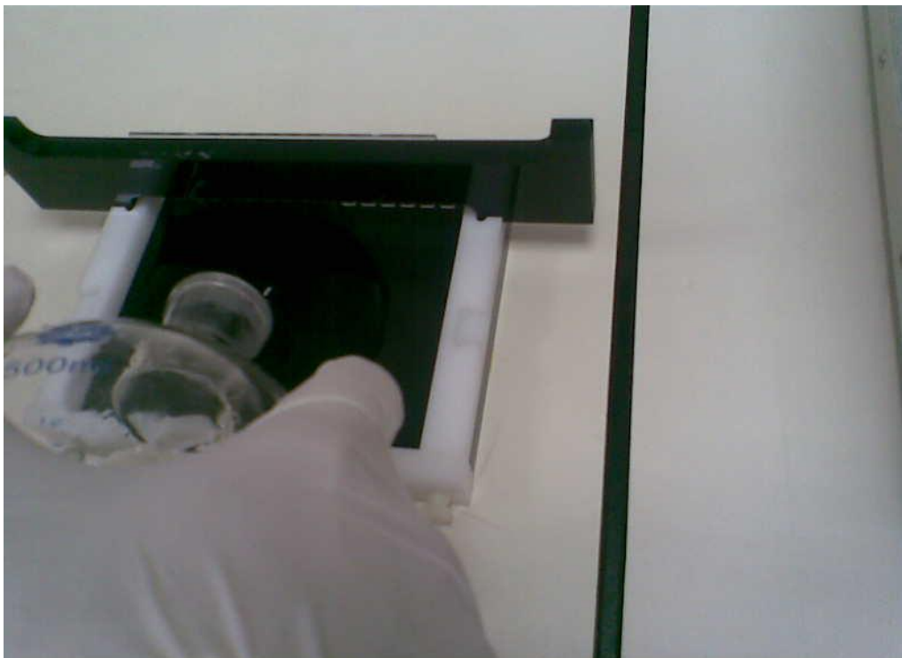
Figure27. Purring Agarose on PFGE frame, (Comb containing samples in Blocks are implanted in gel)
