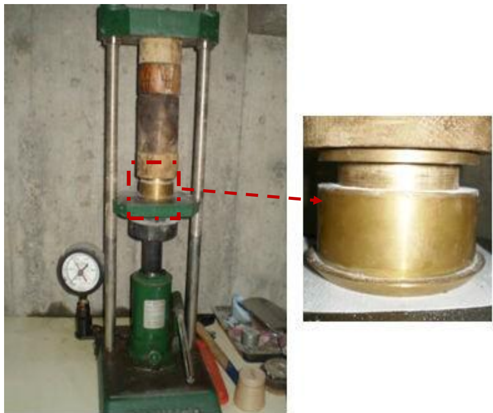
Figure 3.21. A View of Static Compaction by the Help of Hydraulic Jack
