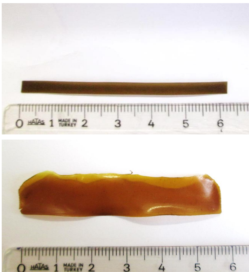
Figure 3.5 Visual appearances of extruded strips before rolling and after rolling
