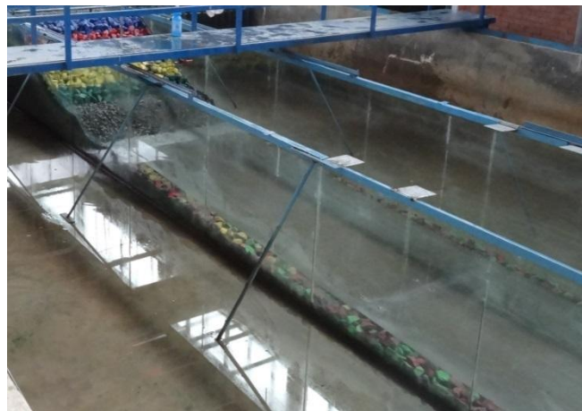
Figure 4.6: 1:30 Slope in the wave channel
