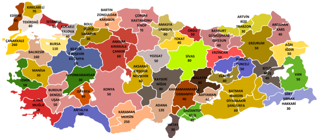
Figure 4-14. Regional Wind Power Connection Capacities declared by TEIAS
