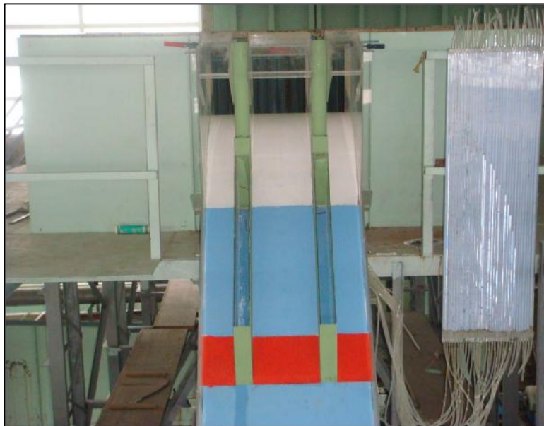
Figure 2.6 The Hydraulic Model with Aeration Ramp (TR-5)
