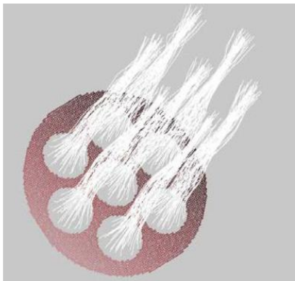
Figure 9 Electron trajectories in a multibeam gun [15]
