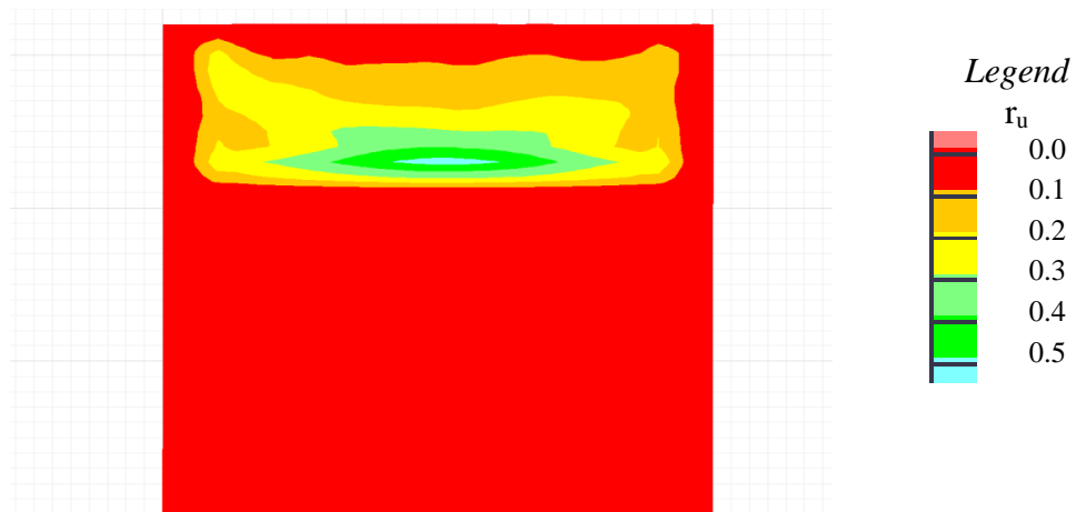
Figure 4.36. Excess pore pressure distribution, r_u , at t=8.0 sec
