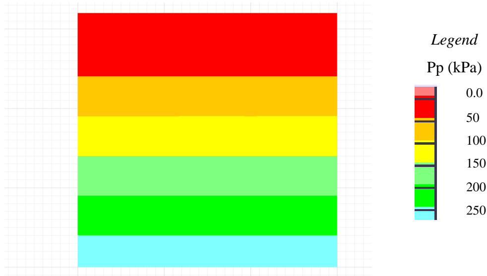
Figure 4.31. Initial Pore Water Pressure Distribution of Port Island Site (kPa)
