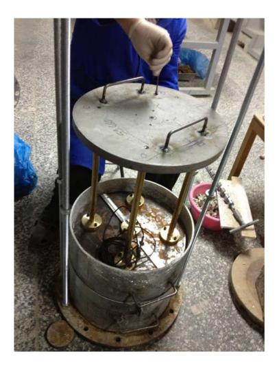
Figure 3.25. Placing load application frame
