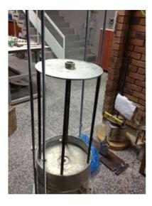
Figure 3.23. Frame for overburden stress
