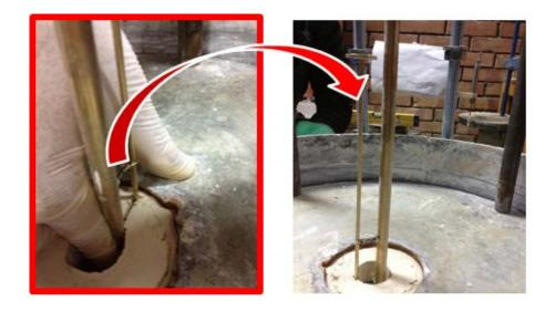
Figure 3.21. Placement of settlement rod
