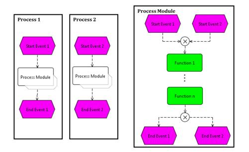
Figure 19 Illustration for usage of process interface construct
