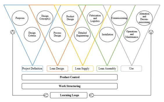
Figure 3.13: Triads of the Lean Project Delivery System with Facility Use (adapted from Koskela et al., 2002)
