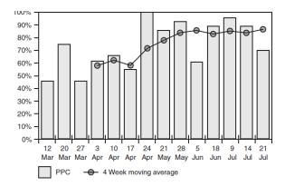
Figure 3.17: Example PPC Chart (Ballard et al., 2002)
