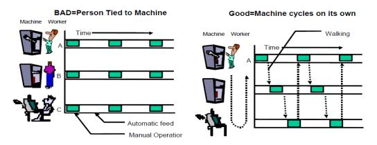
Figure 2.5: Person-Machine Separation (Liker and Lamb, 2000)
