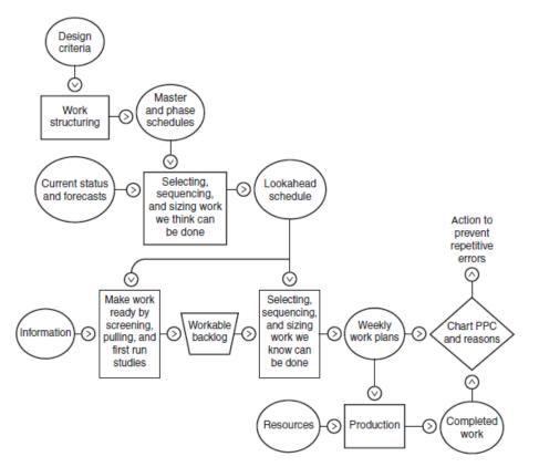
Figure 3.14: Last Planner System of Production Control (Ballard et al., 2002)
