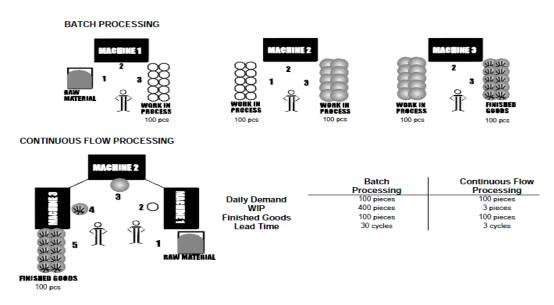
Figure 2.4: Continuous Flow Processing vs. Batch Processing ("Art of Lean")
