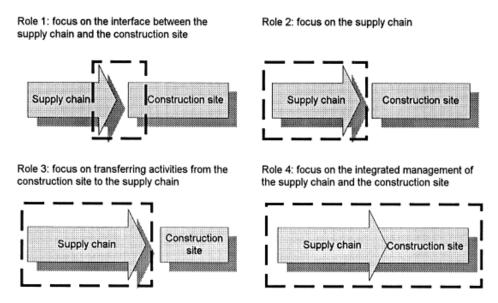
Figure 3.12: The Four Roles of SCM in Construction (Vrijhoef and Koskela, 2000)
