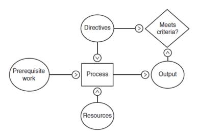
Figure 3.16: Activity Definition Model (Ballard et al., 2002)
