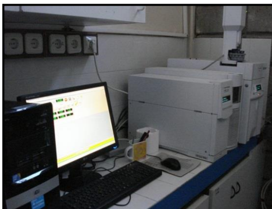
Figure 3.3 Agilent 6850 gas chromatograph (GC) coupled with and Agilent 5975C mass spectrometer (MS).
