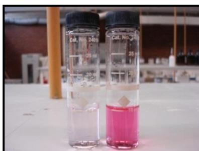
Figure 3.2 Free Chlorine (1 st Sample Cell) & Monochloramine (2 nd Sample Cell)
