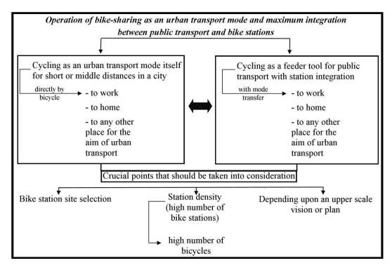
Figure 60. The Relationship between Three Principles of Bike-sharing in Turkey: Bike-sharing as an Urban Transport Mode, Public Transport Integration, and Integration of Planning
