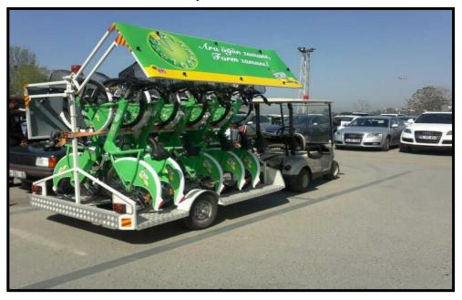
Figure 56. Bicycle maintenance and Reloading Vehicle in İstanbul Bikesharing Systems
