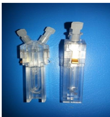
Figure 16. Disposable capillary cell – DTS1060 for zeta potential measurements
