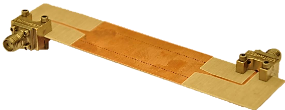
Figure 5-3: Thru line design
