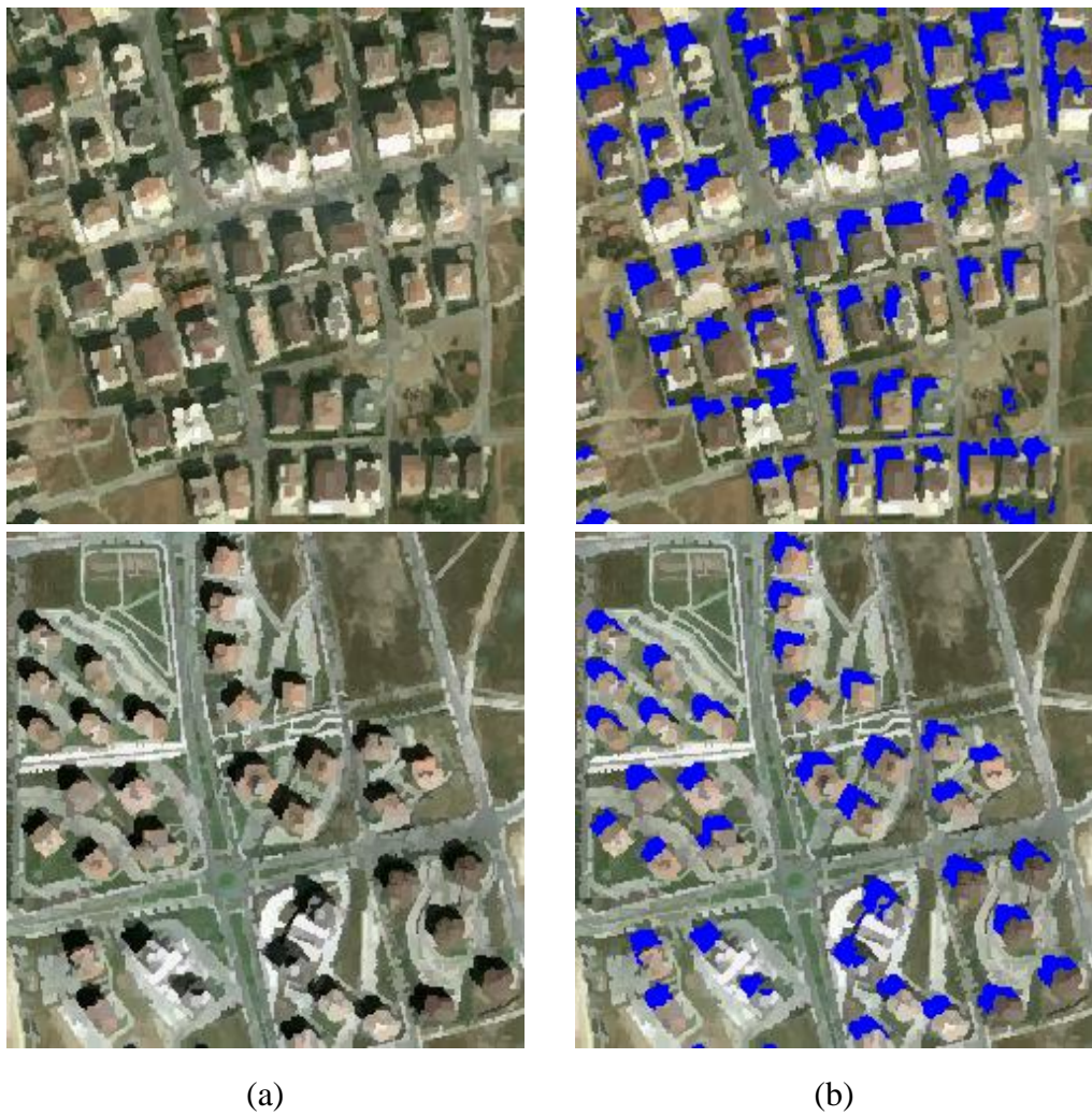
Figure 3.3: Shadow detection example. (a) Over-segmented images. (b) Detected shadows.
