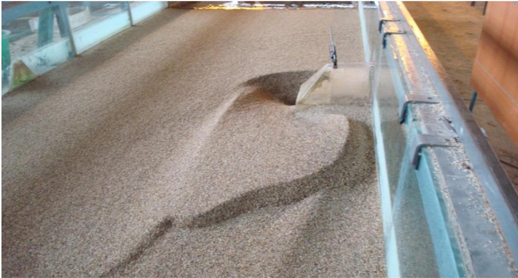
Figure 4-4: Experimental setup with a single abutment configuration.
