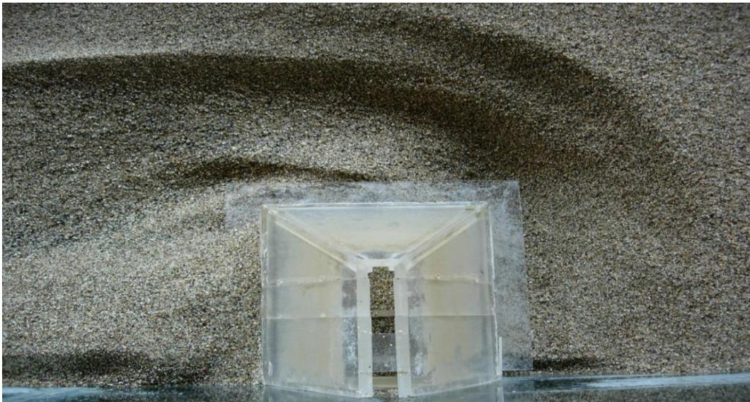
Figure 4-5: Aerial view of sediments around the abutment.
