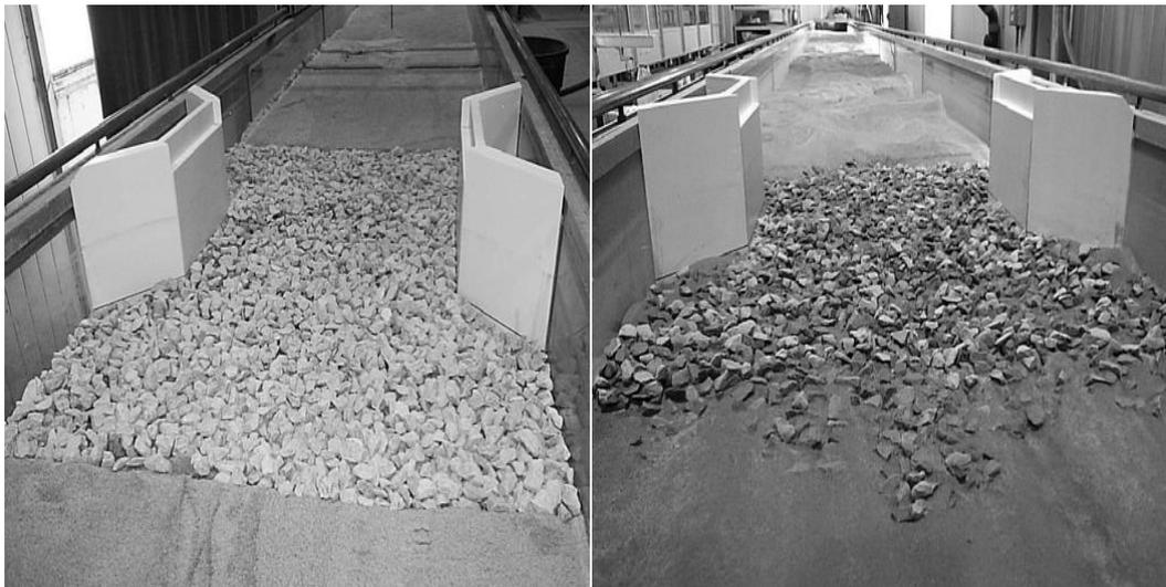
Figure 3-1: Riprap application before and after scour (Barkdoll, Ettema & Melville, 2007).
