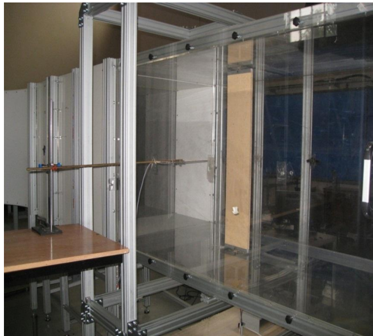
Figure 5.2. Chipboard Blunt Body with Aluminum Ends (Left Side) and Blunt Body Placed in the Wind Tunnel (Right Side)
