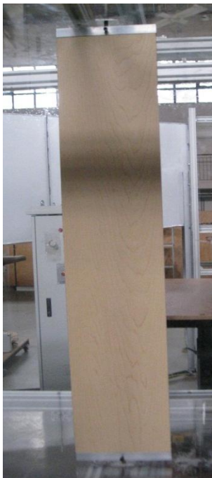
Figure 5.2. Chipboard Blunt Body with Aluminum Ends (Left Side) and Blunt Body Placed in the Wind Tunnel (Right Side)
