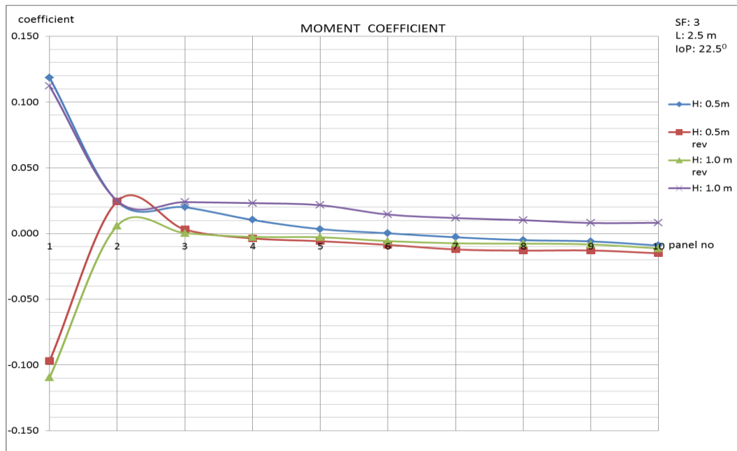
Figure 7.11. Moment Coefficients on Panels for Clear Front Heights H: 0.5 m and 1.0 m
