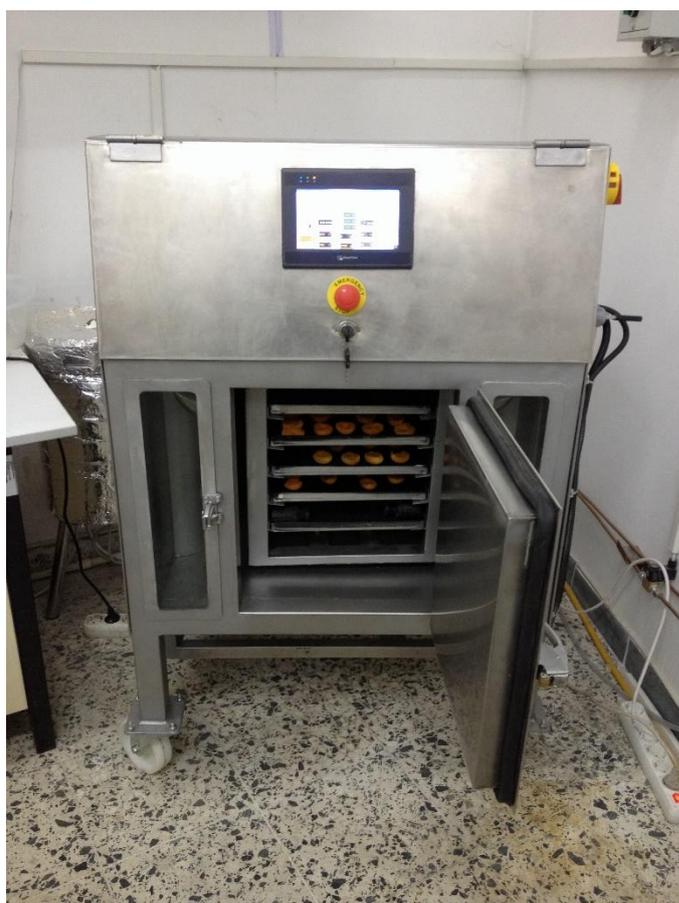
**Figure 3.1** Laboratory scale tray dryer
