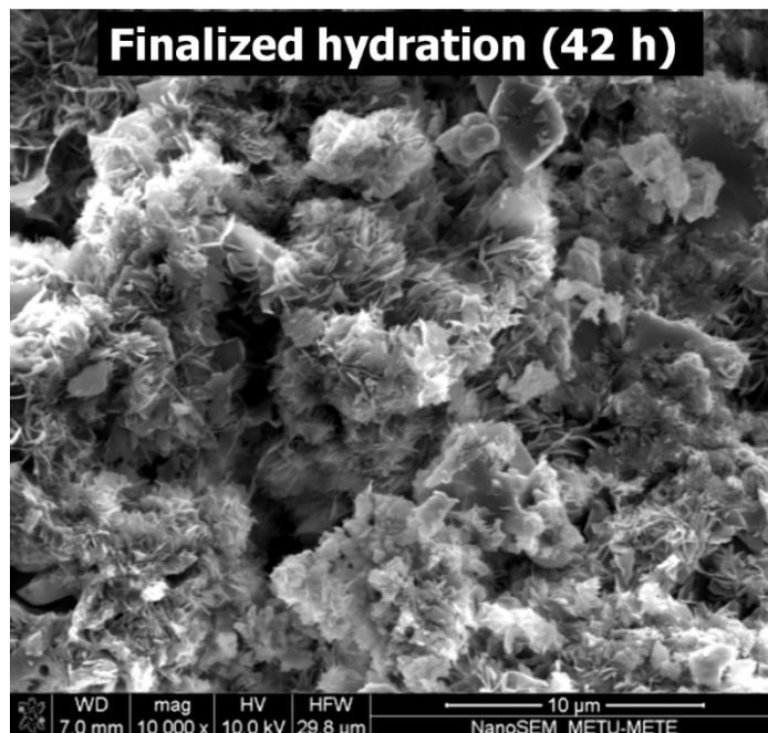
Figure 5.5 SEM micrograph of 42 h hydrated TCP pellet.
