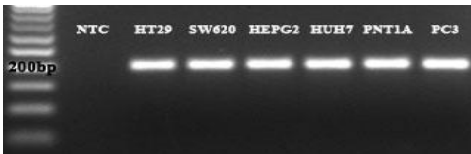
Figure 3.14 qRT-PCR products of GAPDH cDNA (197bp) of each cell line. 5 \mu L of qRT-PCR product was loaded in each well. NTC is the no template control.
