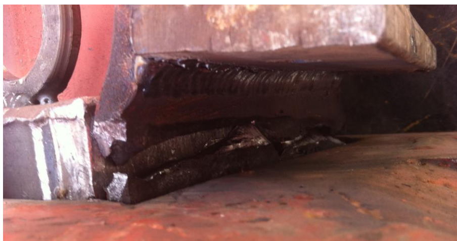
Figure 7.91. Spread Fracture after 97 cycles
