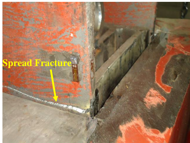
Figure 7.48. Front view of fracture occurs exactly above the 400 mm-high steel base fixture.
