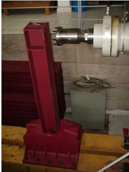
Figure 6.39. HP test specimen mounted onto the stiff steel base fixture.
