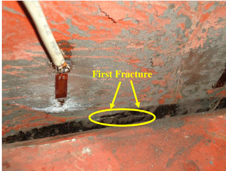
Figure 7.24. First fracture occurs 341 cycles.
