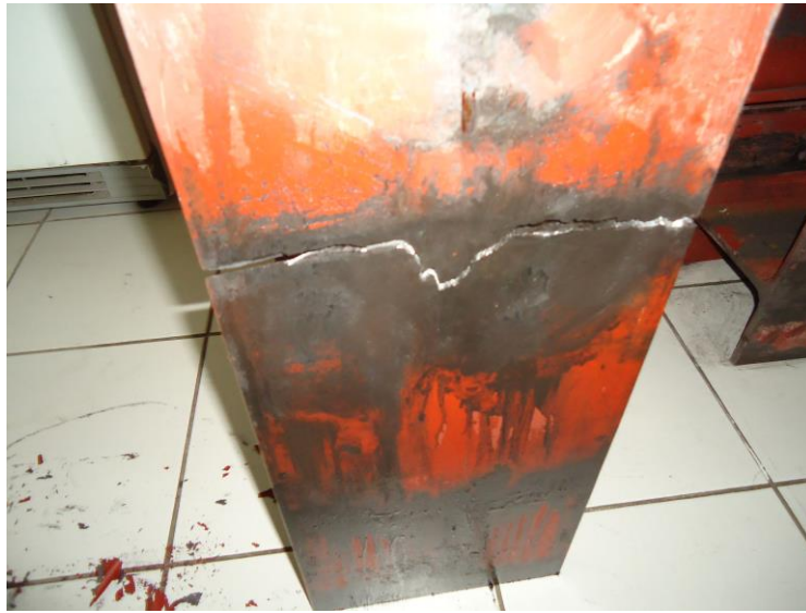
Figure 7.15. Front view of fracture occurs exactly above the 400 mm-high steel base fixture.
