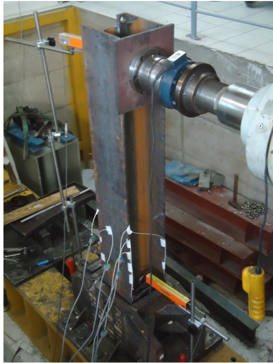
Figure 7.70. Specimen-21 under cyclic lateral load normal to its Weak axis.
