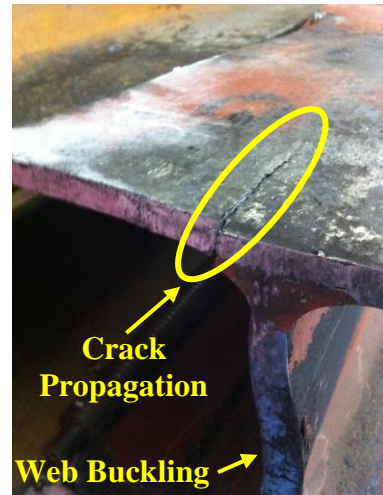
Figure 8.21. (a) Web buckling, (b) Crack propagation
