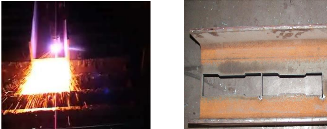
Figure 5.2. Cutting process of standart test speciment with CNC method.
