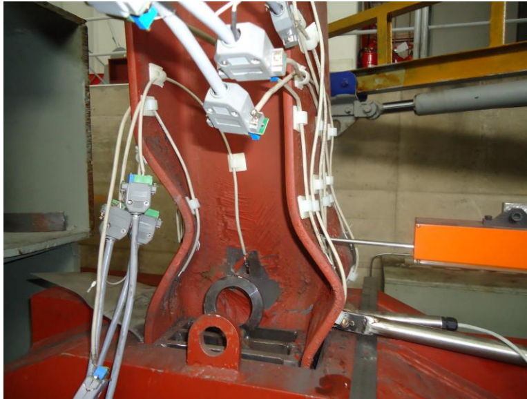
Figure 7.41. Local Buckling in steel HP220x57.
