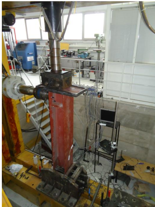
Figure 7.58. Specimen-19 under cyclic lateral and axial load normal to its Strong axis.
