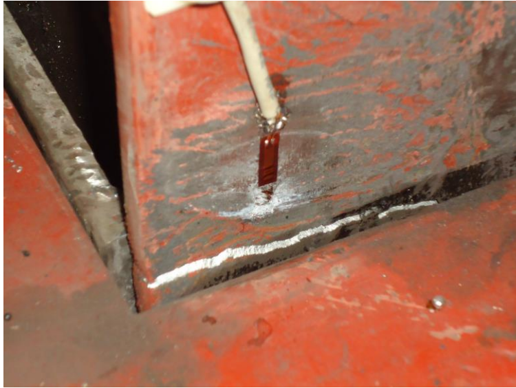
Figure 7.32. Fracture complete after 548 cycles.
