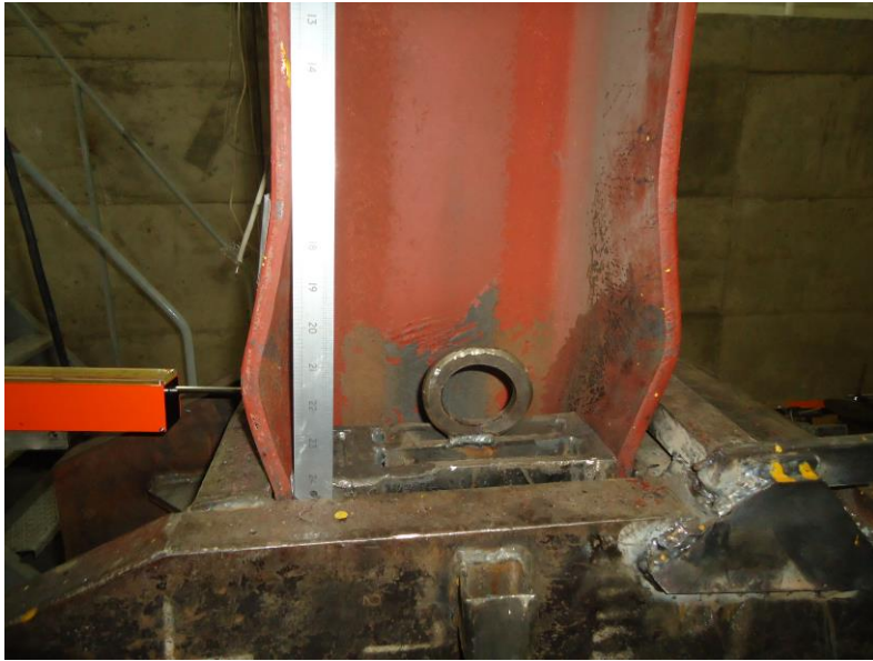
Figure 7.66. Expanding lateral buckling occurring experiment.
