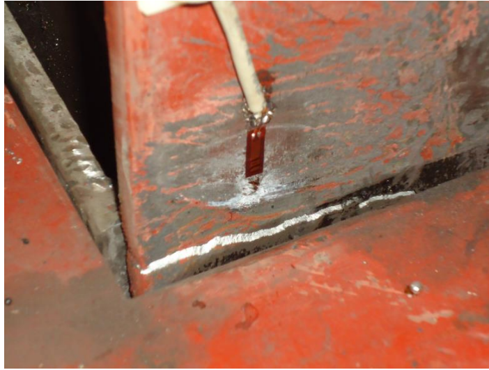
Figure 7.26. Front view of fracture occurs exactly above the 400 mm-high steel base fixture.
