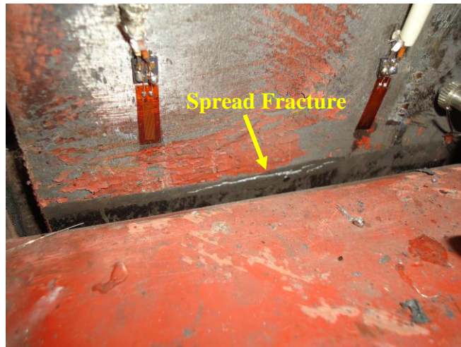
Figure 7.10. First fracture begins expansion after 220 cycles.
