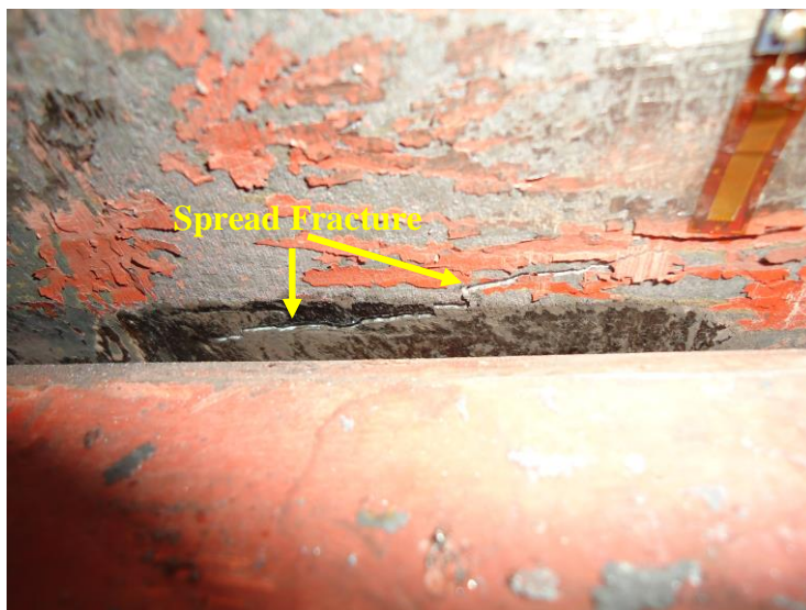
Figure 7.25. First fracture begins expansion after 341 cycles.
