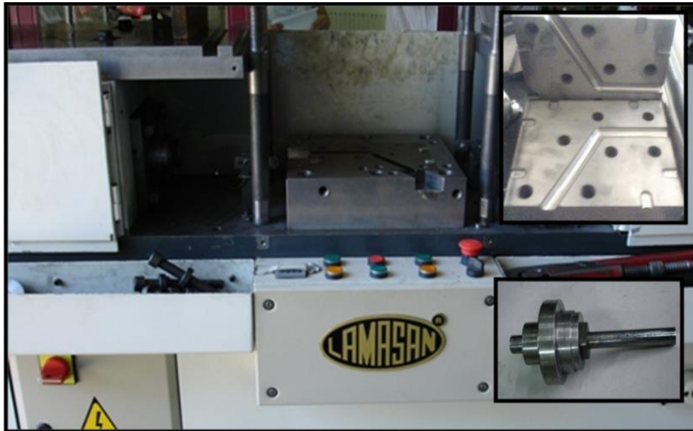
Figure 3.1. ECAP system composed of pressing unit, 120° angle die and 18 mm diameter punch.
