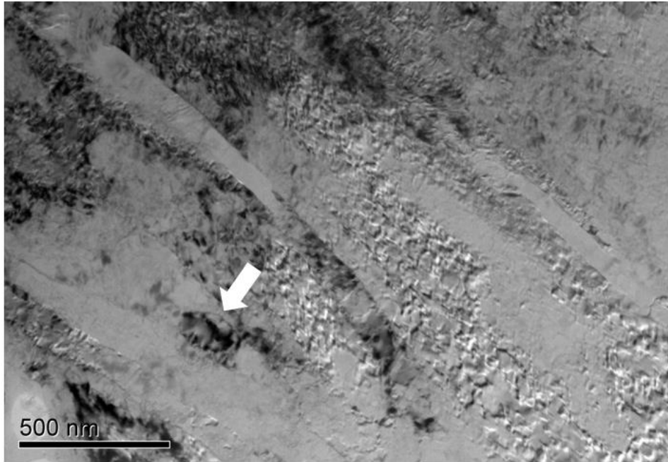
Figure 3.13. TEM images of the ECAPed and over aged Al 2024 (190°C/ 80 min.)
