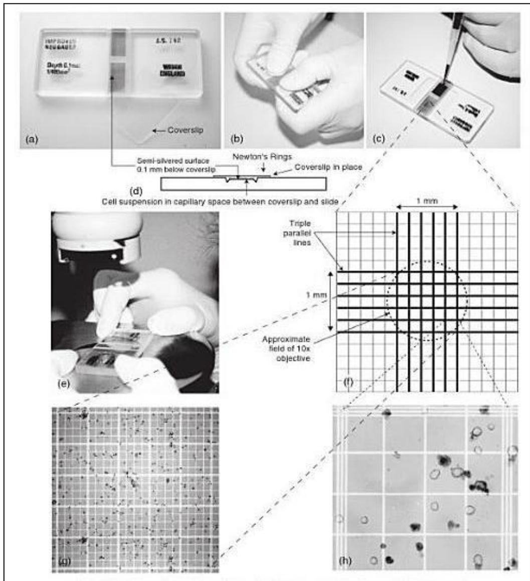
**Figure 2.1.** Hemocytometer chamber (a) showing counting chambers (b) showing coverslip in place (c) showing fill points (d) showing cell suspension in capillary space between coverslip and slide (e) showing inverted phase contrast microscope and close up of a counting square
