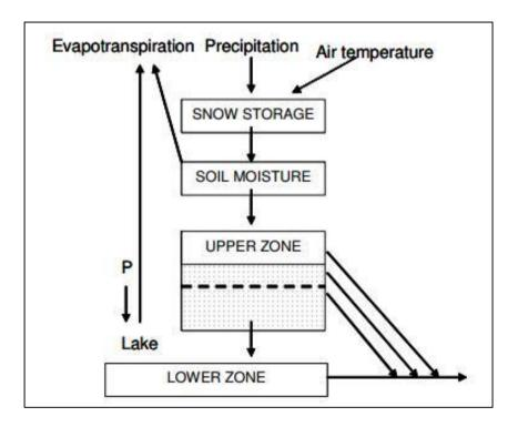
Figure 4.1 The HBV model structure: storage zones and main fluxes (Lawrence et al. 2009).
