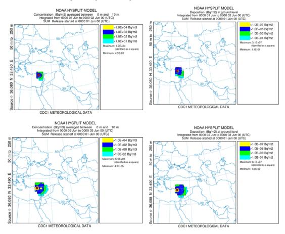
Figure 4.11. Atmospheric Dispersion Graphs of HYSPLIT for Hypothetical Accident at Akkuyu NPP
