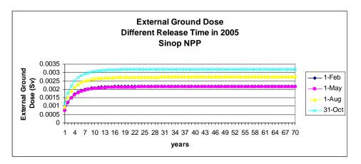
Figure 4.25. External Ground Doses for the Releases Starting on Different Times in 2005 for the Hypothetical Accident at Sinop NPP
