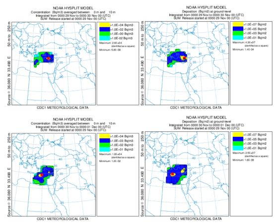
Figure B.1. Atmospheric Dispersion Graphs of HYSPLIT for Hypothetical Accident at Akkuyu NPP
