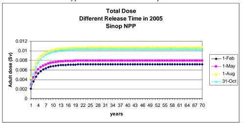
Figure 4.27. Total Dose Incurred for the Releases Starting on Different Times in 2005 for the Hypothetical Accident at Sinop NPP
