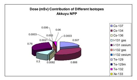
**Figure B.11.** Dose Contribution of the Different Isotopes for Akkuyu NPP Accident Case Study (Release started on 29<sup>th</sup> of November 2000)
