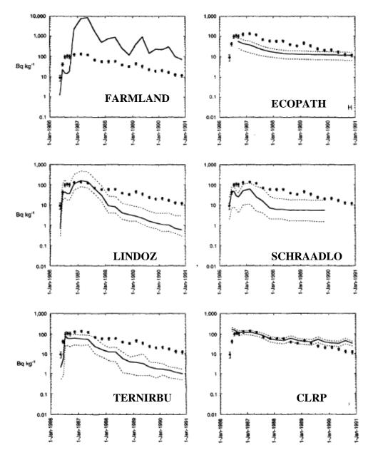
**Figure 4.5.** Average Concentrations in Beef Predicted by Different Models Vertical bars indicate 95% confidence intervals on the mean value of observations (dark circles); dashed lines indicate the 95% subjective confidence interval about the mean prediction (solid line).
