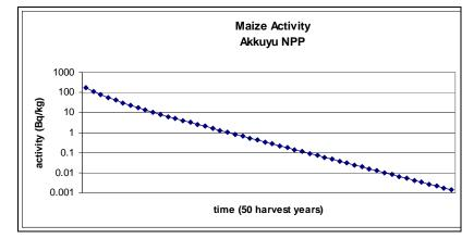
Figure B.7. Activity in Maize for for Hypothetical Accident at Akkuyu NPP
